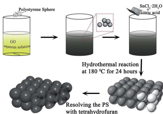
Fig. 1 A schematic representation of the synthesis process.
