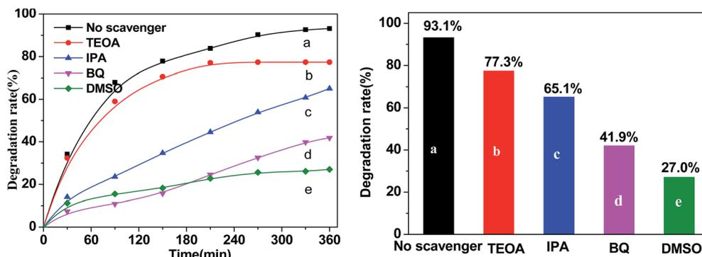
Fig. 12 Photocatalytic degradation ratios of TC-HCl by  $\text{Fe}_3\text{O}_4/\text{rGO}/\text{TiO}_2$  using different radical scavengers (a) reaction in the absence of radical scavengers, (b) reaction with 100 mM TEOA as a scavenger for  $\text{h}^+$ , (c) reaction with 100 mM IPA for  $\cdot\text{OH}$ , and (d) reaction with 0.2 mM BQ for  $\cdot\text{O}_2^-$  (e) reaction with 100 mM DMSO as a scavenger for  $\text{e}^-$  under visible light irradiation for 360 min.
