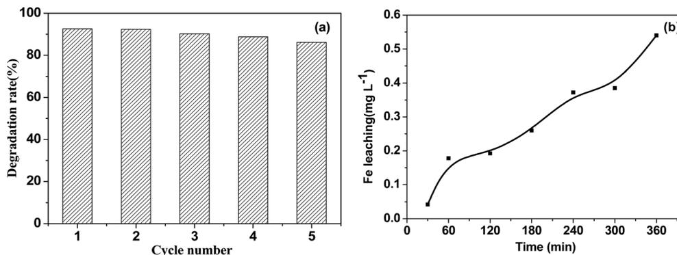
Fig. 10 (a) The stability of the  $\text{Fe}_3\text{O}_4/\text{rGO}/\text{TiO}_2$  photocatalyst for the discoloration of TC-HCl (b) the Fe leaching from  $\text{Fe}_3\text{O}_4/\text{rGO}/\text{TiO}_2$  photocatalyst in the first cycle as a function of time.
