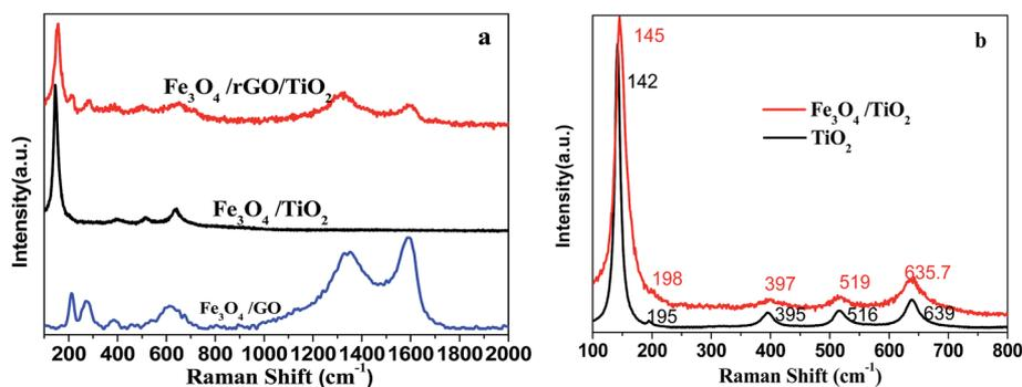
Fig. 4 Raman spectra of (a)  $\text{Fe}_3\text{O}_4/\text{TiO}_2$ ,  $\text{Fe}_3\text{O}_4/\text{GO}$ ,  $\text{Fe}_3\text{O}_4/\text{rGO}/\text{TiO}_2$  nanocomposite (b) detail information of the Raman spectra of  $\text{TiO}_2$  and  $\text{Fe}_3\text{O}_4/\text{TiO}_2$  nanocomposite.
