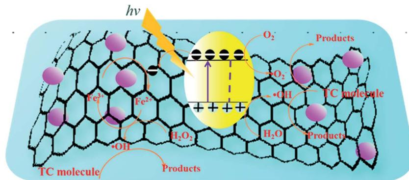
Fig. 13 Proposed schematic illustration showing the reaction mechanism for photocatalytic degradation of TC-HCl over the  $\text{Fe}_3\text{O}_4/\text{rGO}/\text{TiO}_2$  nanocomposites in which pink spheres, yellow oval and black sheet represent  $\text{Fe}_3\text{O}_4$  nanoparticles,  $\text{TiO}_2$  nanoparticles and rGO, respectively.
