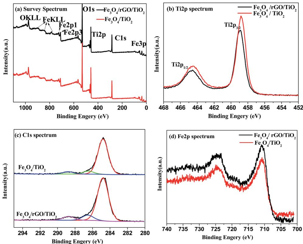
Fig. 6 XPS spectra of  $\text{Fe}_3\text{O}_4/\text{TiO}_2$  and  $\text{Fe}_3\text{O}_4/\text{rGO}/\text{TiO}_2$  nanocomposite: (a) full spectra of samples; (b) Ti 2p peaks; (c) C 1s peaks; (d) Fe 2p peaks.
