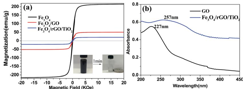
Fig. 3 (a) Magnetic hysteresis curves of  $\text{Fe}_3\text{O}_4$  nanoparticles,  $\text{Fe}_3\text{O}_4/\text{GO}$  and  $\text{Fe}_3\text{O}_4/\text{rGO}/\text{TiO}_2$  nanocomposite (inset: separation of particles dispersed in water by a magnet in 1 min). (b) UV-vis absorbance of GO and  $\text{Fe}_3\text{O}_4/\text{rGO}/\text{TiO}_2$  nanocomposite.
