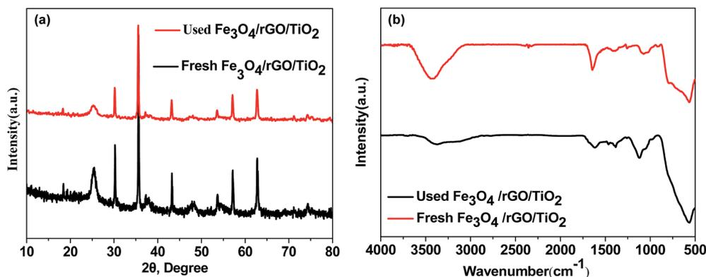
Fig. 11 (a) XRD pattern and (b) FT-IR spectra of the pristine and used  $\text{Fe}_3\text{O}_4/\text{rGO}/\text{TiO}_2$  photocatalyst.
