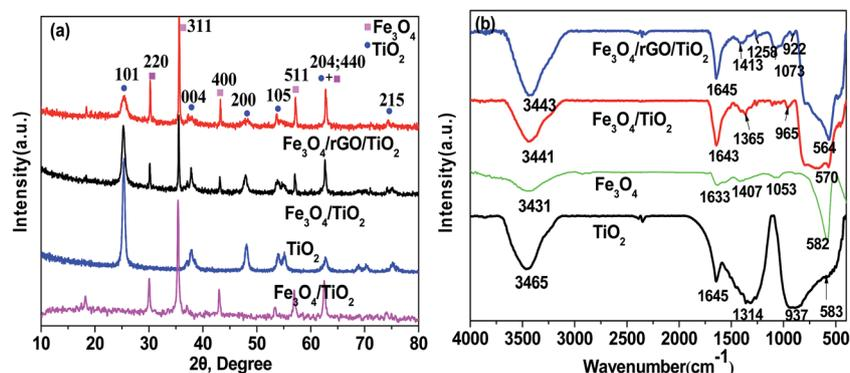
Fig. 2 XRD patterns (a) and FTIR spectra (b) of  $\text{Fe}_3\text{O}_4$ , anatase  $\text{TiO}_2$ ,  $\text{Fe}_3\text{O}_4/\text{TiO}_2$  and  $\text{Fe}_3\text{O}_4/\text{rGO}/\text{TiO}_2$ . The blue spheres (●) and pink cubes (■) indicate the typical diffraction peaks of anatase  $\text{TiO}_2$  and  $\text{Fe}_3\text{O}_4$ , respectively.
