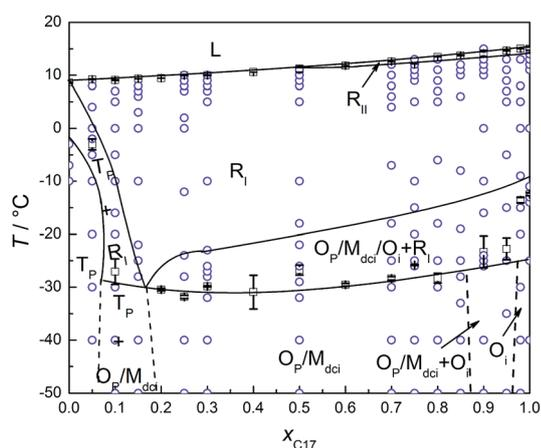
Fig. 4 Phase transition temperature of  $\text{C}_{16}$ – $\text{C}_{17}$  binary system confined in CPG (8.1 nm) as a function of mole fraction of  $x_{\text{C}_{17}}$ , estimated using DSC ( $\square$ ) and temperature-dependent XRD ( $\circ$ ) in the heating processes. The dotted lines were estimated from the diffraction results.
