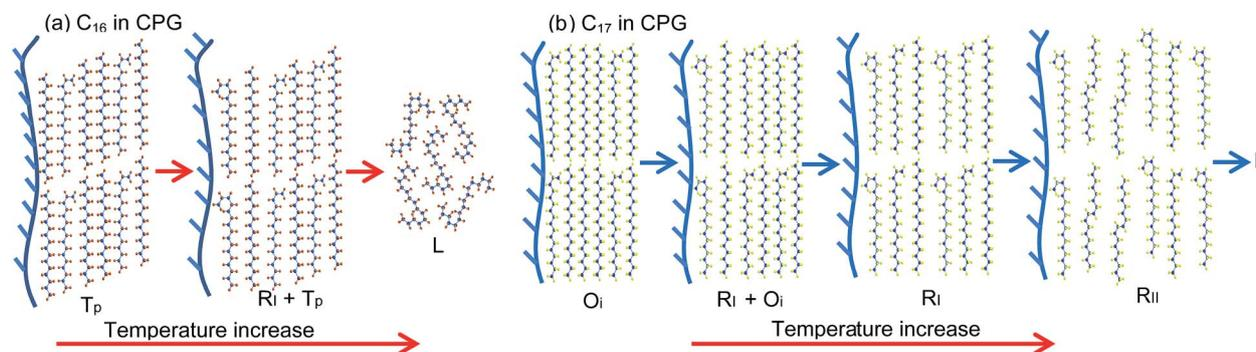
Fig. 8 Possible structural transformations of  $C_{16}$  from  $T_{16}$  in bulk to [ $R_I + T_{16}$ ] and melt confined in CPG (8.1 nm) (a), and  $C_{17}$  from  $O_{17}$  in bulk to [ $R_I + O_{17}$ ],  $R_I$ , and  $R_{II}$  phase confined in CPG (8.1 nm) (b).
