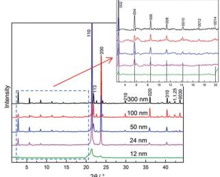
Fig. 6 Reflection patterns of C $_{23}$  in CPG (nominal d=12-300 nm) recorded at room temperature ( $\sim$ 24  $^{\circ}$ C) in the low temperature phase, orthorhombic O $_{1}$  (O $_{23}$ ), together with the vertical lines of from the standard PDF card of C $_{23}$ .
