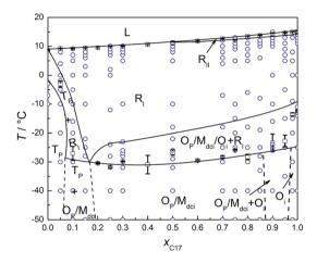
Fig. 4 Phase transition temperature of  $C_{16}-C_{17}$  binary system confined in CPG (8.1 nm) as a function of mole fraction of  $x_{C_{12}}$ , estimated using DSC (
