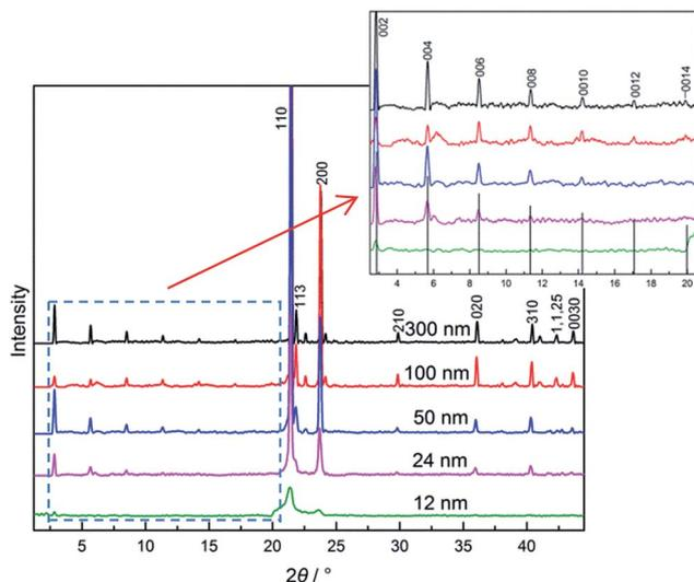
Fig. 6 Reflection patterns of  $C_{23}$  in CPG (nominal  $d = 12\text{--}300$  nm) recorded at room temperature ( $\sim 24^\circ\text{C}$ ) in the low temperature phase, orthorhombic  $O_i$  ( $O_{23}$ ), together with the vertical lines of from the standard PDF card of  $C_{23}$ .
