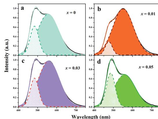
Fig. 6 Emission spectra fit to two Gaussian functions show the contribution to the emission spectra from  $Eu^{2+}$  in two distinct crystallographic sites. Dashed lines represent the individual Gaussian functions and the solid line represents the total fit.
