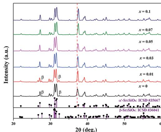
Fig. 1 XRD patterns of  $\text{Sr}_{1.98}\text{Si}_{1-x}\text{Al}_x\text{O}_{4-2x}\text{N}_x:0.02\text{Eu}$  ( $x = 0-0.1$ ), together with the standard data for  $\alpha'/\beta\text{-Sr}_2\text{SiO}_4$  (ICSD #35667 and ICSD #36041) as reference.
