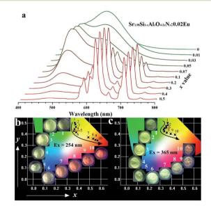
Fig. 4 (a) PL spectra ( $\lambda_{ex} = 320 \text{ nm}$ ) of  $Sr_{1.98}Si_{1-x}Al_xO_{4-2x}N_x:0.02Eu$ (x = 0-0.5). (b & c) Dependence of CIE chromaticity coordinates and digital photos on various x values upon 254 and 365 nm excitation, respectively. The numbers 1-10 corresponds to the x values from 0 to 0.5.
