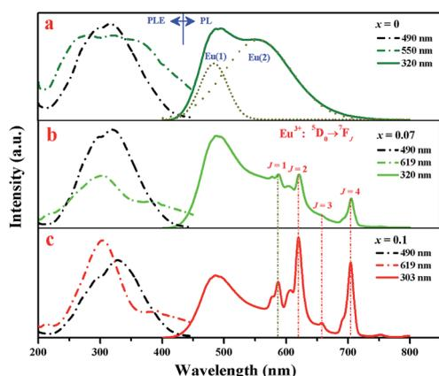
Fig. 3 Room-temperature PLE and PL spectra of  $\text{Sr}_{1.98}\text{Si}_{1-x}\text{Al}_x\text{O}_{4-2x}\text{N}_x:0.02\text{Eu}$  ( $x = 0, 0.07$  and  $0.1$ ) phosphors.
