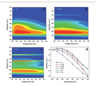
Fig. 7 (a–c) Temperature-dependent (300–460 K) PL spectra contour plots for  $\mathrm{Sr}_{1.98}\mathrm{Si}_{1-x}\mathrm{Al}_x\mathrm{O}_{4-2x}\mathrm{N}_x$ :0.02Eu (x=0, 0.07 and 0.1) excited at 320 nm; (d) dependence of integrated PL intensities on measured temperature for samples  $\mathrm{Sr}_2\mathrm{Si}_{1-x}\mathrm{Al}_x\mathrm{O}_{4-2x}\mathrm{N}_x$ :0.02Eu (x=0-0.2).
