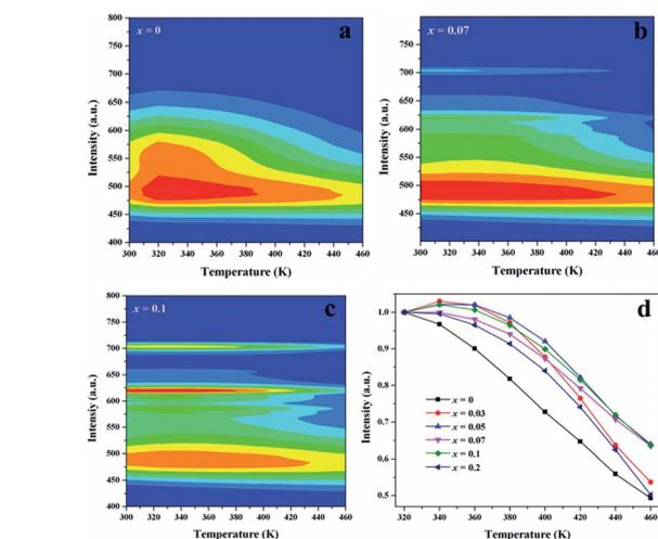
Fig. 7 (a–c) Temperature-dependent (300–460 K) PL spectra contour plots for  $\text{Sr}_{1.98}\text{Si}_{1-x}\text{Al}_x\text{O}_{4-2x}\text{N}_x:0.02\text{Eu}$  ( $x = 0, 0.07$  and  $0.1$ ) excited at 320 nm; (d) dependence of integrated PL intensities on measured temperature for samples  $\text{Sr}_2\text{Si}_{1-x}\text{Al}_x\text{O}_{4-2x}\text{N}_x:0.02\text{Eu}$  ( $x = 0-0.2$ ).
