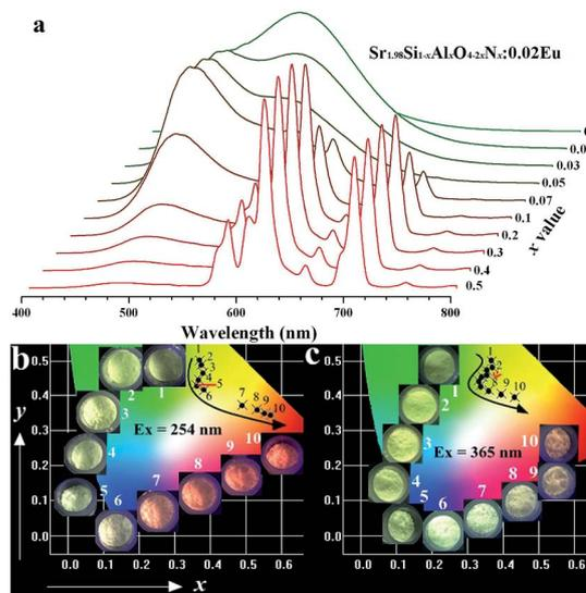
Fig. 4 (a) PL spectra ( $\lambda_{ex} = 320$  nm) of Sr<sub>1.98</sub>Si<sub>1-x</sub>Al<sub>x</sub>O<sub>4-2x</sub>N<sub>x</sub>:0.02Eu ( $x = 0-0.5$ ). (b & c) Dependence of CIE chromaticity coordinates and digital photos on various  $x$  values upon 254 and 365 nm excitation, respectively. The numbers 1–10 corresponds to the  $x$  values from 0 to 0.5.
