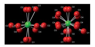
Fig. 2 Coordination spheres of the two different  $\mathrm{Sr}^{2+}$  sites in the disordered  $\alpha'$ -Sr<sub>2</sub>Si<sub>1-x</sub>Al<sub>x</sub>O<sub>4-2x</sub>N<sub>x</sub>.
