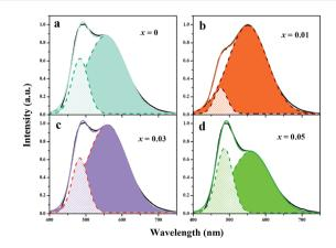
Fig. 6 Emission spectra fit to two Gaussian functions show the contribution to the emission spectra from Eu<sup>2+</sup> in two distinct crystallographic sites. Dashed lines represent the individual Gaussian functions and the solid line represents the total fit.
