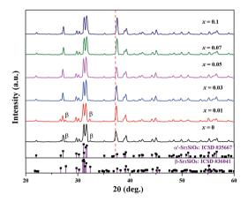
Fig. 1 XRD patterns of  $Sr_{1.98}Si_{1.-x}Al_xO_{4-2x}N_x$ :0.02Eu (x=0-0.1), together with the standard data for  $\alpha'/\beta$ - $Sr_2SiO_4$  (ICSD #35667 and ICSD #36041) as reference.
