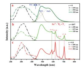
Fig. 3 Room-temperature PLE and PL spectra of  $Sr_{1.98}Si_{1-x}Al_xO_{4-2x}$  $N_x$ : 0.02Eu (x = 0, 0.07 and 0.1) phosphors.
