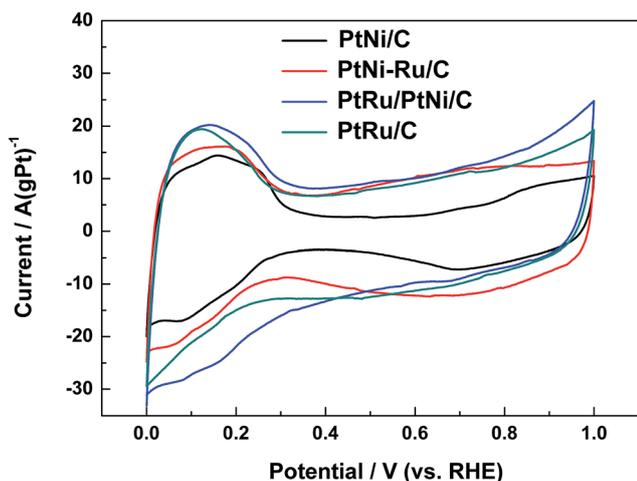
Fig. 5 CVs of different catalysts in 0.1 mol L<sup>-1</sup> HClO<sub>4</sub> solution at a scan rate of 20 mV s<sup>-1</sup>.
