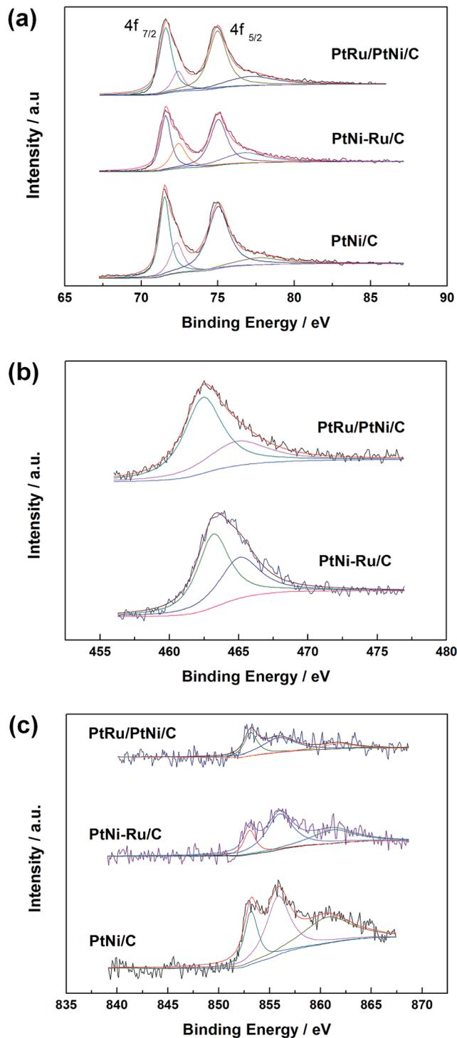
Fig. 4 XPS spectra of Pt 4f (a), Ru 3p<sub>3/2</sub> (b) and Ni 2p<sub>3/2</sub> (c) in PtNi/C, PtNi–Ru/C and PtRu/PtNi/C catalysts.
