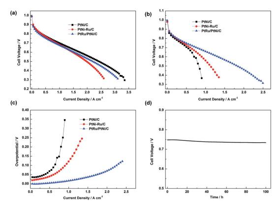
Fig. 7 Curves of cell voltage vs. current density of PEMFC fed with  $H_2$  (a) and  $H_2/30$  ppm CO mixture (b). (c) CO overpotential of PtNi/C, PtNi-Ru/ C and PtRu/PtNi/C catalysts under different current density. (d) Single cell stability test of the PtRu/PtNi/C catalyst fed with H<sub>2</sub>/30 ppm CO mixture at 0.5 A cm<sup>-2</sup>
