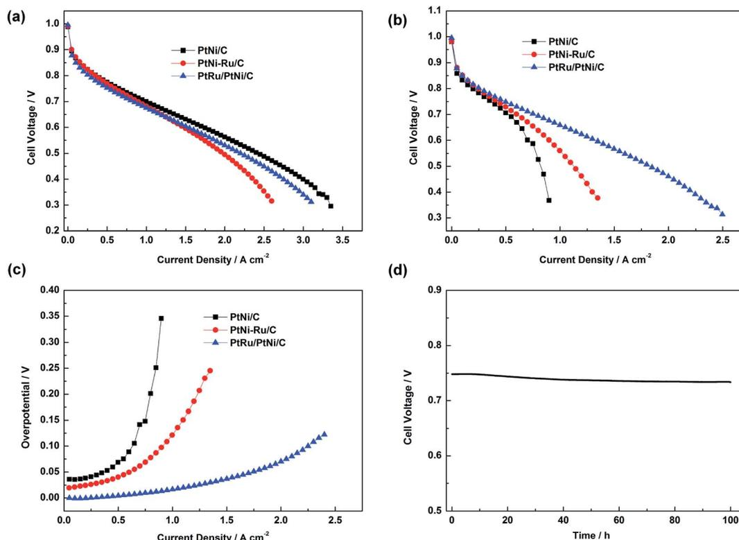
Fig. 7 Curves of cell voltage vs. current density of PEMFC fed with H<sub>2</sub> (a) and H<sub>2</sub>/30 ppm CO mixture (b). (c) CO overpotential of PtNi/C, PtNi-Ru/C and PtRu/PtNi/C catalysts under different current density. (d) Single cell stability test of the PtRu/PtNi/C catalyst fed with H<sub>2</sub>/30 ppm CO mixture at 0.5 A cm<sup>-2</sup>.
