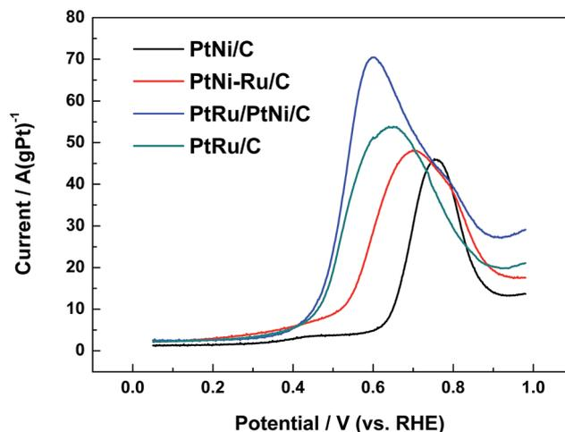
Fig. 6 CO stripping voltammograms of different catalysts in 0.1 mol L<sup>-1</sup> HClO<sub>4</sub> solution at a scan rate of 20 mV s<sup>-1</sup>.
