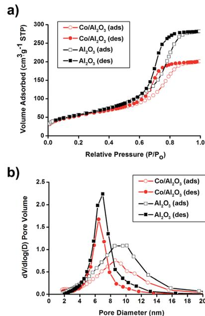
**Fig. 2** (a) N<sub>2</sub> adsorption/desorption isotherms and (b) pore size distribution diagrams of pristine Al<sub>2</sub>O<sub>3</sub> and Co/Al<sub>2</sub>O<sub>3</sub> nanocatalyst.
