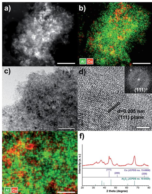
**Fig. 1** (a) HADDF-TEM image, (b) low-resolution scanning-TEM image with elemental mapping of cobalt and aluminium, (c) TEM image, (d) HR-TEM image with the corresponding Fourier-transform pattern (inset of d), (e) magnified scanning-TEM image, and (f) XRD spectrum of Co/Al<sub>2</sub>O<sub>3</sub> nanocatalyst. The bars represent 200 nm (a, b), 100 nm (c), 2 nm (d), and 10 nm (e).
