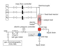
Fig. 3 Schematic diagram of Fischer-Tropsch synthesis reaction instruments.
