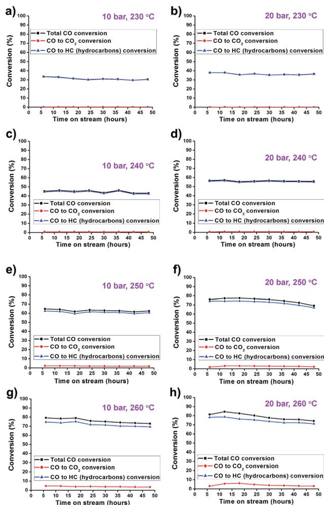
Fig. 4 (a–h) CO conversion graphs of Co/Al<sub>2</sub>O<sub>3</sub> nanocatalyst at 10–20 bar and 230–260 °C. The total CO conversion is the sum of the CO conversion to hydrocarbons (CO to HC) and the CO conversion to CO<sub>2</sub> (CO to CO<sub>2</sub>). The reaction tests were conducted at GHSV = 6.8 NL g<sub>cat</sub><sup>-1</sup> h<sup>-1</sup> and a H<sub>2</sub> : CO ratio of '2'.
