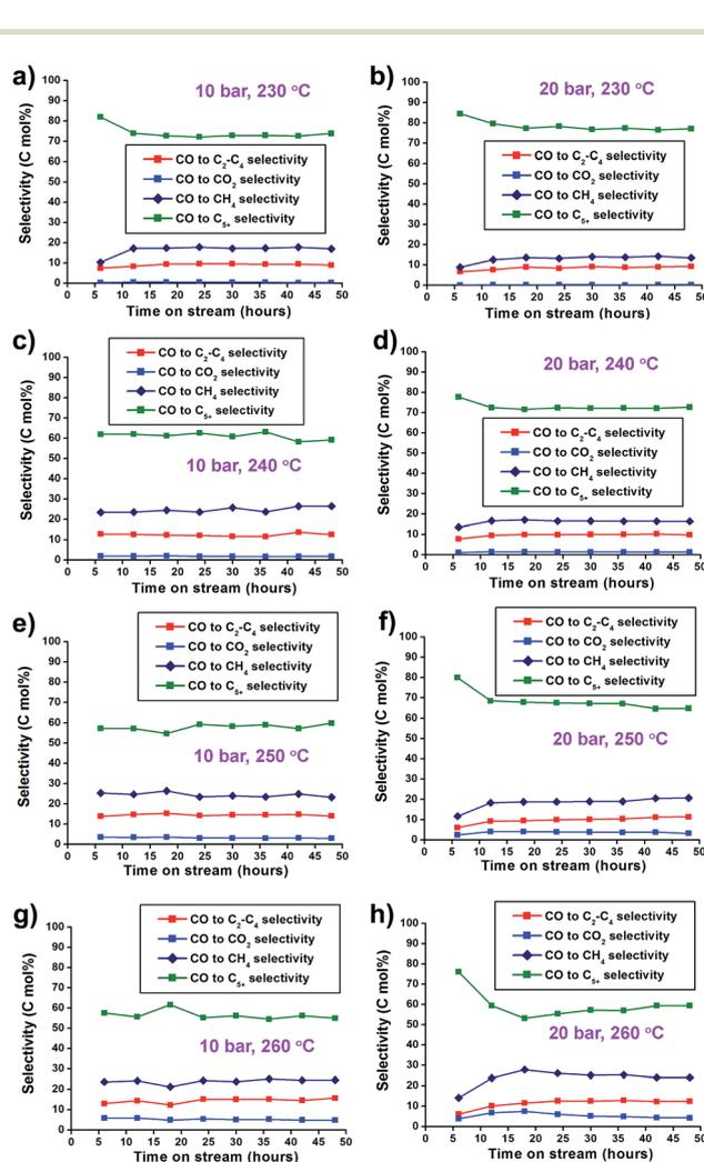
Fig. 5 (a–h) CO<sub>2</sub> and hydrocarbon selectivity graphs of Co/Al<sub>2</sub>O<sub>3</sub> nanocatalyst at 10–20 bar and 230–260 °C. The reaction tests were conducted at GHSV = 6.8 NL g<sub>cat</sub><sup>-1</sup> h<sup>-1</sup> and a H<sub>2</sub> : CO ratio of '2'.
