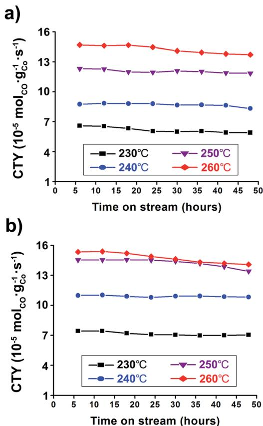
Fig. 6 Cobalt-Time-Yield (CTY) graphs conducted under 230–260 °C at (a) 10 bar and (b) 20 bar. The reaction tests were conducted at GHSV = 6.8 NL g<sub>cat</sub><sup>-1</sup> h<sup>-1</sup> and a H<sub>2</sub> : CO ratio of '2'.
