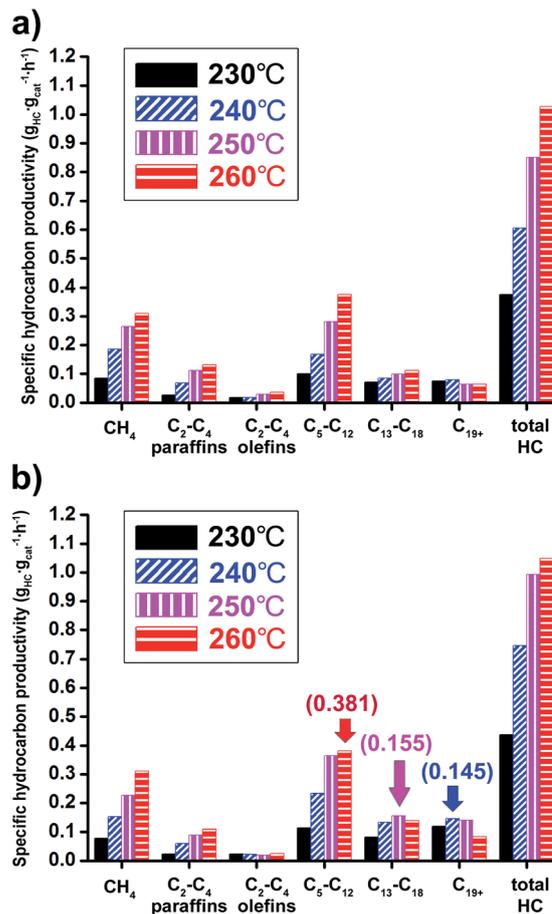
Fig. 7 Hydrocarbon productivity data of Co/Al<sub>2</sub>O<sub>3</sub> nanocatalyst conducted under 230–260 °C at (a) 10 bar and (b) 20 bar. The reaction tests were conducted at GHSV = 6.8 NL g<sub>cat</sub><sup>-1</sup> h<sup>-1</sup> and a H<sub>2</sub> : CO ratio of '2'.
