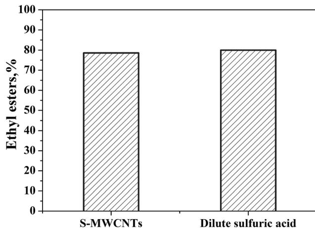
Fig. 5 Ethyl ester yield using S-MWCNTs and 0.5 mol L<sup>-1</sup> sulfuric acid as catalysts at the same condition.
