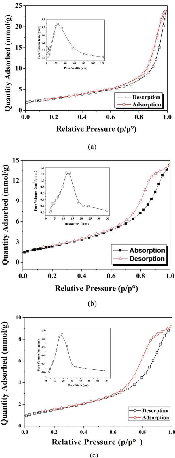
Fig. 1 The N<sub>2</sub> adsorption–desorption isotherms and pore size distributions of the studied catalysts: (a) MWCNT, (b) new S-MWCNTs and (c) after the first use S-MWCNTs.
