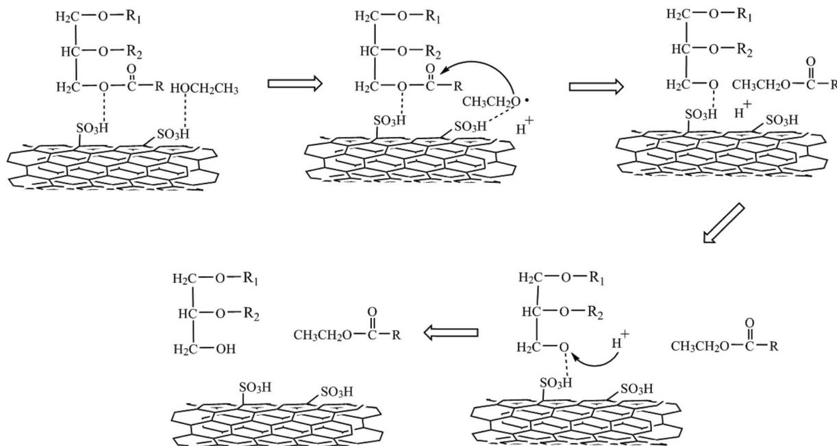
Fig. 10 The proposed mechanism for the transesterification reaction in ethanol on S-MWCNTs.
