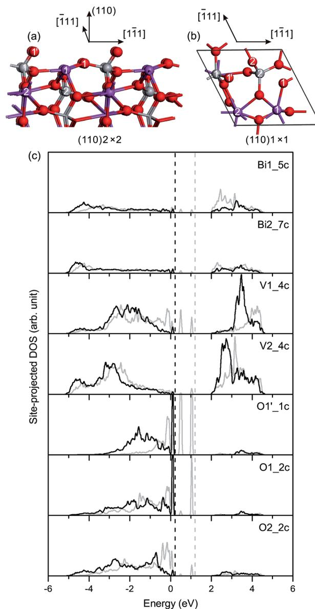
Fig. 6 (a) Side view and (b) top view of the relaxed geometric structure of the fm-BiVO<sub>4</sub> (110) surface. (c) Site-projected DOS of specific surface atoms in the relaxed and unrelaxed (110) surface slabs, denoted by black and grey, respectively.
