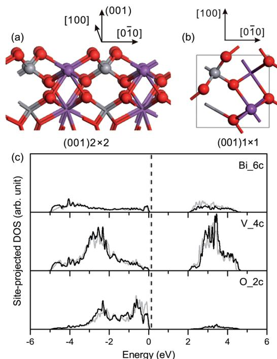
**Fig. 4** (a) Side view and (b) top view of the relaxed geometric structure of the fm-BiVO<sub>4</sub> (001) surface. (c) Site-projected DOS of specific surface atoms in the relaxed and unrelaxed (001) surface slabs, denoted by black and grey, respectively.
