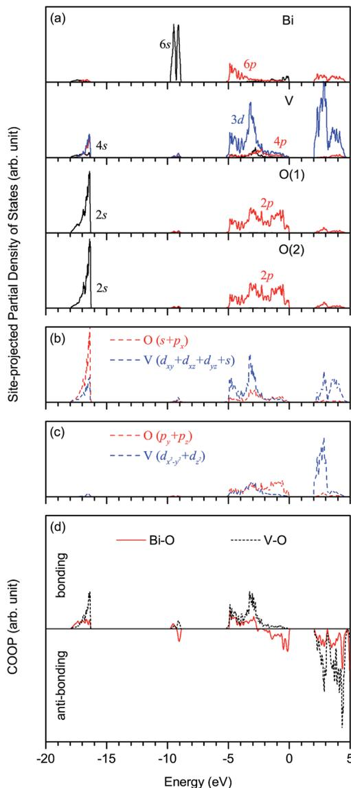
**Fig. 2** Site-projected partial density of states of fm-BiVO<sub>4</sub>: (a) for s, p and d orbitals of Bi, V, O(1) and O(2) atoms, (b) for V ( $d_{xy} + d_{xz} + d_{yz} + s$ ) and O ( $s + p_x$ ) hybrid orbitals, and (c) for V ( $d_{z^2} + d_{x^2-y^2}$ ) and O ( $p_y + p_z$ ) orbitals. (d) COOP curves for the Bi–O and V–O bonds. The Fermi level is at zero energy.
