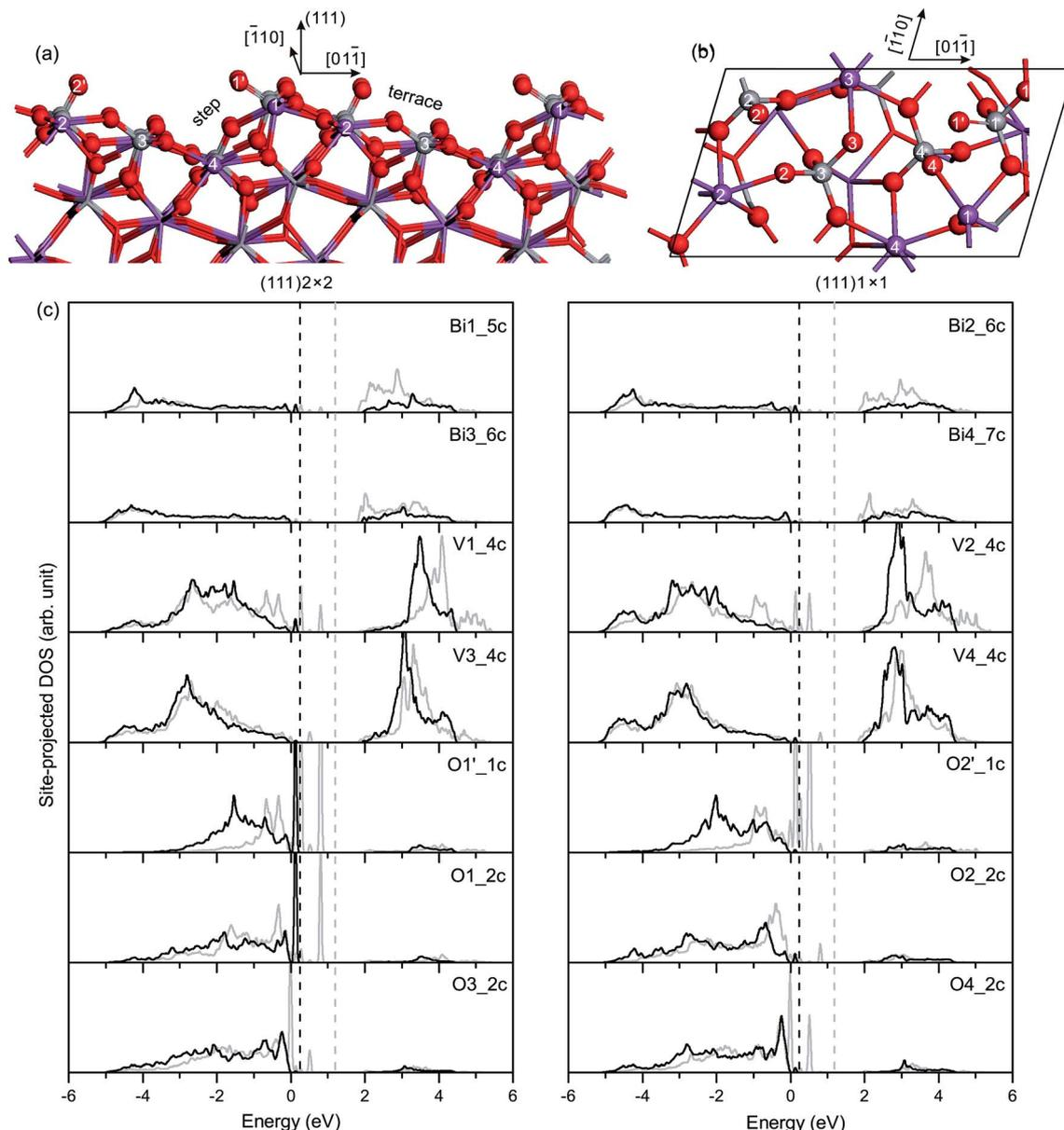
Fig. 7 (a) Side view and (b) top view of the relaxed geometric structure of the fm-BiVO<sub>4</sub> (111) surface. (c) Site-projected DOS of specific surface atoms in the relaxed and unrelaxed (111) surface slabs, denoted by black and grey, respectively.
