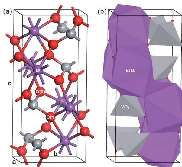
**Fig. 1** Crystal structure of fm-BiVO<sub>4</sub>. (a) In the ball-stick model and (b) in the polyhedron model. The Bi, Ti and O atoms are in purple, gray and red, respectively.
