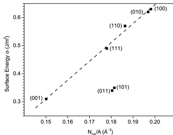
Fig. 8 The relaxed surface energy  $\sigma_r$  vs. surface density of disrupted Bi–O bonds  $N_{\text{DB}}/A$  for low-index surfaces of fm-BiVO<sub>4</sub>.
