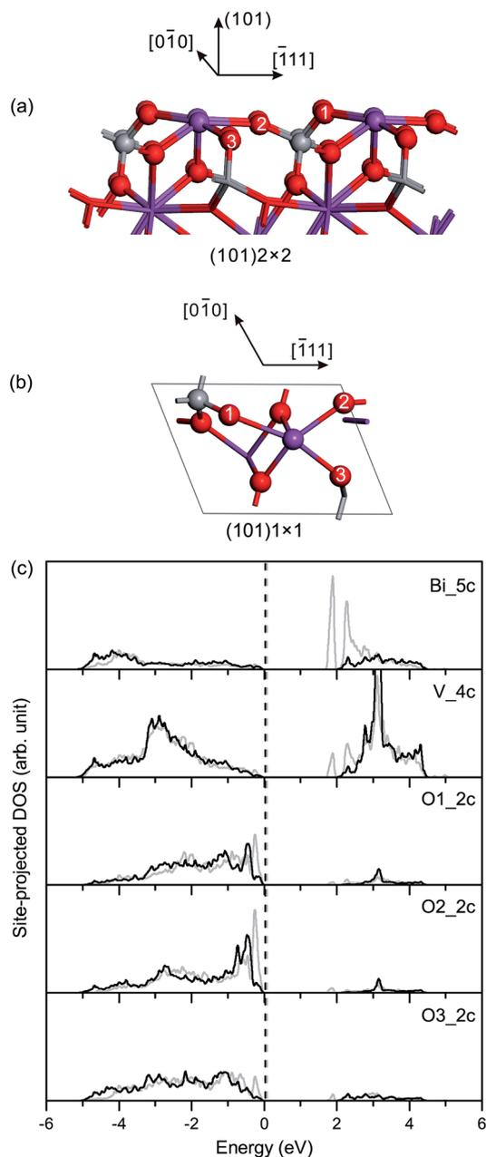
Fig. 5 (a) Side view and (b) top view of the relaxed geometric structure of the fm-BiVO<sub>4</sub> (101) surface. (c) Site-projected DOS of specific surface atoms in the relaxed and unrelaxed (101) surface slabs, denoted by black and grey, respectively.
