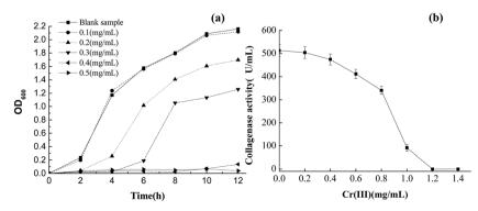
Tolerance curves of (a) B. amyloliquefaciens TCCC11319 for Cr(III) concentration and (b) collagenase for Cr(III) concentration.
