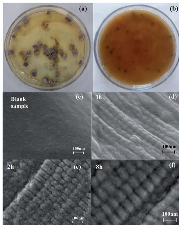
Fig. 6 Degradation of CTLS by enzyme produced from *B. amyloliquefaciens* TCCC11319. (a) Initial CTLS. (b) CTLS hydrolyzed for 24 h. FESEM images of (c) CTLS, (d) hydrolyzed CTLS within 1 h, (e) hydrolyzed CTLS within 2 h, and (f) hydrolyzed CTLS within 8 h.
