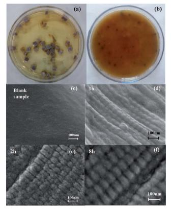
Fig. 6 Degradation of CTLS by enzyme produced from *B. amyloli-quefaciens* TCCC11319. (a) Initial CTLS. (b) CTLS hydrolyzed for 24 h. FESEM images of (c) CTLS, (d) hydrolyzed CTLS within 1 h, (e) hydrolyzed CTLS within 2 h, and (f) hydrolyzed CTLS within 8 h.
