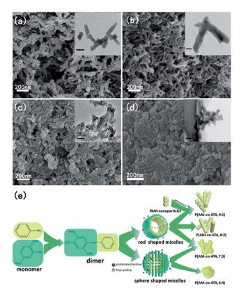
Fig. 2 SEM images of P(ANI-co-ATA, 9:1) (a), P(ANI-co-ATA, 8:2) (b), P(ANI-co-ATA, 7:3) (c) and P(ANI-co-ATA, 6:4) (d). The insets in each SEM images are the corresponding TEM images of copolymers with the scale bar represents 50 nm. (e) The proposed growth mechanism for copolymers synthesized at different ANI/ATA values.
