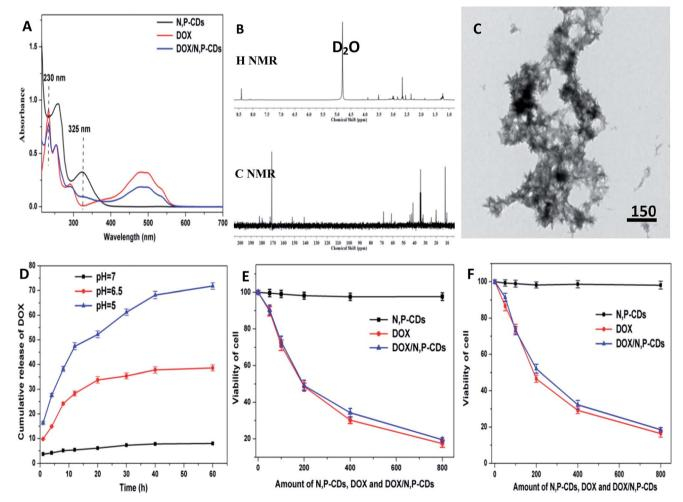
Fig. 4 (A) UV-vis absorption spectra of N,P-CDs, DOX, and DOX/N,P-CDs. (B)  $^1$ H-NMR and  $^{13}$ C-NMR of DOX/N,P-CDs. (C) TEM image of DOX/N,P-CDs. Scale bar = 200 nm. (D) DOX release profile from the DOX/N,P-CD prodrug at 37  $^{\circ}$ C. (E) Cytotoxicity evaluation of N,P-CDs, DOX, and DOX/N,P-CDs towards A549 cells after 48 h culturing. (F) Cytotoxicity evaluation of N,P-CDs, DOX, and DOX/N,P-CDs towards HeLa cells after 48 h culturing.
