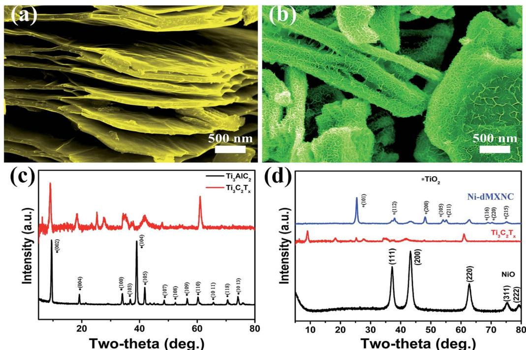
Fig. 1 SEM images of the (a) as-obtained  $\text{Ti}_3\text{C}_2\text{T}_x$  MXene after DMSO treatment, and (b) the as-obtained Ni-dMXNC. (c) XRD patterns of pre-HF-treated  $\text{Ti}_3\text{AlC}_2$  MAX phase and post-HF treated  $\text{Ti}_3\text{C}_2\text{T}_x$  MXene. (d) XRD patterns of NiO nanosheets,  $\text{Ti}_3\text{C}_2\text{T}_x$  MXene, and Ni-dMXNC.
