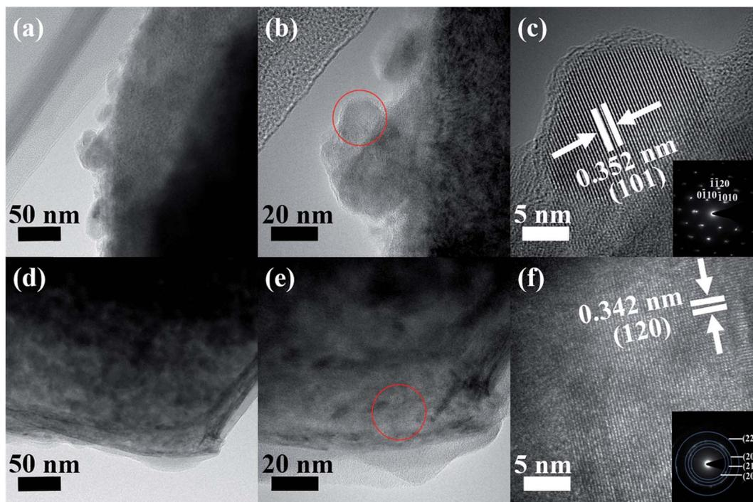
Fig. 4 (a) and (b) Low-magnification TEM image, (c) HRTEM image (red circle area in (b)), and corresponding SAED pattern (inset) of the  $\text{Ti}_3\text{C}_2\text{T}_x$  MXene; (d) and (e) low-magnification TEM image, (f) HRTEM image (red circle area in (e)), and corresponding SAED pattern (inset) of the Ni-dMXNC.
