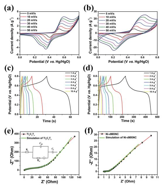
Fig. 5 CV curves of the (a)  $T_{13}C_2T_x$  and (b) Ni-dMXNC electrodes at various scan rates; GCD curves of the (c)  $T_{13}C_2T_x$  and (d) Ni-dMXNC electrodes at various scan rates and current densities. EIS of the (e)  $T_{13}C_2T_x$  and (f) Ni-dMXNC electrodes.
