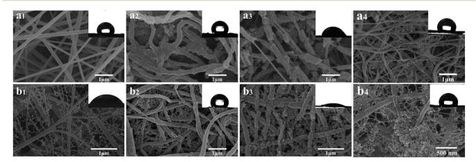
Fig. 1 FE-SEM images of (a1) PVDF, (a2) PVDF-PPy, (a3) PVDF-PPy-MnO<sub>2</sub>, (a4) PVDF-MnO<sub>2</sub>, (b1) PVDF/TBAC, (b2) PVDF/TBAC-PPy, (b3) PVDF/TBAC-PPy-MnO<sub>2</sub> and (b4) PVDF/TBAC-MnO<sub>2</sub> nanofiber mat (insert: contact angle of nanofiber mat).
