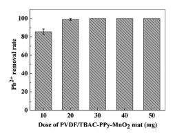
Fig. 7 Effect of PVDF/TBAC-PPy-MnO<sub>2</sub> nanofiber mat dose on the Pb<sup>2+</sup> removal performance.
