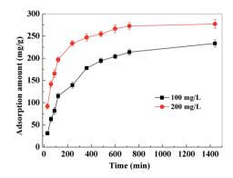
Fig. 9 Effect of contact time and initial concentration on the adsorption of Pb<sup>2+</sup> by PVDF/TBAC-PPy-MnO<sub>2</sub> nanofiber mat.
