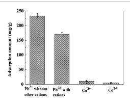
Fig. 14 Effect of coexisting metal ions on the Pb<sup>2+</sup> adsorption.
