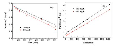
Fig. 10 Pseudo-first-order kinetic model (a), pseudo-second-order kinetic model (b) for adsorption of Pb2+ onto PVDF/TBAC-PPy-MnO2 nanofiber mat.
