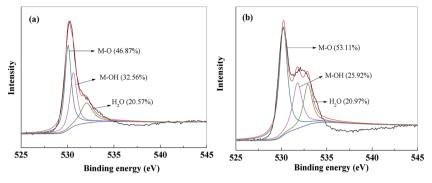
Fig. 17 XPS spectra of O 1s of PVDF/TBAC-PPy-MnO<sub>2</sub> nanofiber mat before (a) and after (b) Pb<sup>2+</sup> adsorption
