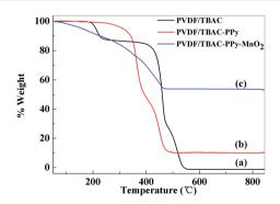
Fig. 3 Thermo-gravimetric curves for (a) PVDF/TBAC, (b) PVDF/TBAC-PPy and (c) PVDF/TBAC-PPy-MnO  $_{\rm 2}$  nanofiber mat.
