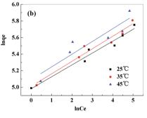
Fig. 12 Langmuir isotherm model (a), Freundlich isotherm model (b) for adsorption of Pb<sup>2+</sup> onto PVDF/TBAC-PPy-MnO<sub>2</sub> nanofiber mat.
