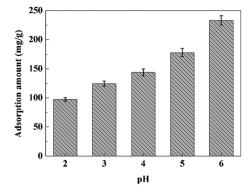
Fig. 8 Effect of pH on the removal of Pb<sup>2+</sup> by the PVDF/TBAC-PPy-MnO<sub>2</sub> nanofiber mat.
