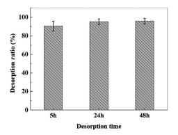
Fig. 16 Desorption efficiency of different desorption time for lead-loaded PVDF/TBAC-PPy-MnO<sub>2</sub> nanofiber mat.
