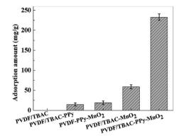
Fig. 4 The adsorption amount of Pb<sup>2+</sup> by different adsorbents.
