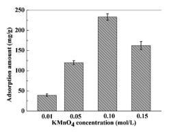
Fig. 6 The adsorption amount of PVDF/TBAC-PPy-MnO<sub>2</sub> nanofiber mat obtained from different KMnO<sub>4</sub> concentrations.
