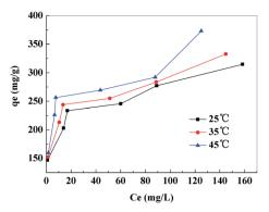
Fig. 11 Equilibrium isotherms of Pb<sup>2+</sup> onto PVDF/TBAC-PPy-MnO<sub>2</sub> nanofiber mat.
