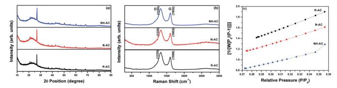
Fig. 1 (a) X-ray diffraction patterns, (b) Raman spectra and (c) surface area plots of unannealed activated carbon (R-AC) and activated carbon annealed under an  $N_2$  atmosphere (N-AC) and annealed under an  $N_3$  atmosphere (NH-AC).
