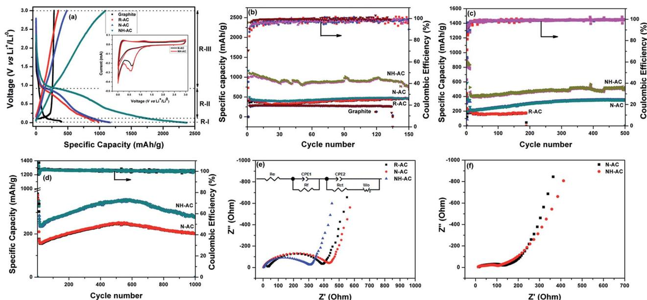
**Fig. 4** Electrochemical performance of R-AC, N-AC, and NH-AC: (a) first discharge–charge plots at 50 mA g<sup>-1</sup> (with inset containing cyclic voltammograms of N-AC and NH-AC obtained at a scan rate of 0.1 mV s<sup>-1</sup> for 3 cycles each); specific capacity plots at (b) 50 mA g<sup>-1</sup>, (c) 200 mA g<sup>-1</sup>, and (d) 500 mA g<sup>-1</sup>; and impedance spectra and equivalent circuit (inset) of N-AC and NH-AC electrodes (e) before cycling and (f) after 1000 cycles.
