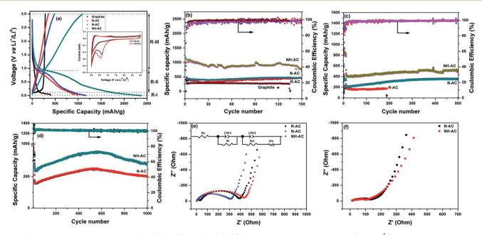
Fig. 4 Electrochemical performance of R-AC, N-AC, and NH-AC: (a) first discharge-charge plots at 50 mA g<sup>-1</sup> (with inset containing cyclic voltammograms of N-AC and NH-AC obtained at a scan rate of 0.1 mV s<sup>-1</sup> for 3 cycles each); specific capacity plots at (b) 50 mA g<sup>-1</sup>, (c) 200 mA g<sup>-1</sup>, and (d) 500 mA g<sup>-1</sup>; and impedance spectra and equivalent circuit (inset) of N-AC and NH-AC electrodes (e) before cycling and (f) after 1000 cycles.
