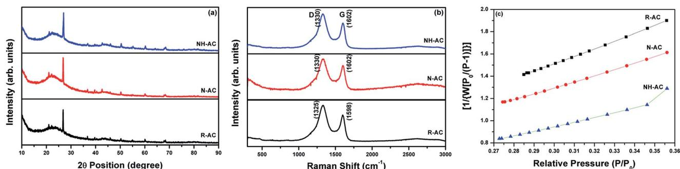
Fig. 1 (a) X-ray diffraction patterns, (b) Raman spectra and (c) surface area plots of unannealed activated carbon (R-AC) and activated carbon annealed under an  $\text{N}_2$  atmosphere (N-AC) and annealed under an  $\text{NH}_3$  atmosphere (NH-AC).
