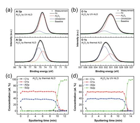
Fig. 3 High resolution XPS spectra for the (a) Al 2p, (b) O 1s core level of Al<sub>2</sub>O<sub>3</sub> thin films by thermal ALD and UV-ALD at 40 °C. XPS depth profiles for the Al<sub>2</sub>O<sub>3</sub> thin film grown at 40 °C by (c) thermal ALD and (d) UV-ALD
