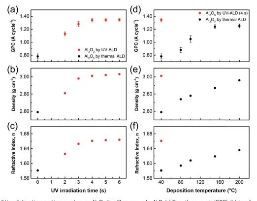
Fig. 2 Effect of UV irradiation time and temperature on  $Al_2O_3$  thin films grown by ALD. (a) Growth per cycle (GPC), (b) density, and (c) refractive index of the film grown at 40 °C as a function of UV irradiation time (2 s in  $H_2O$  dosing step and 0–4 s for additional exposure in purging step); (d) GPC, (e) density, and (f) refractive index of the film as a function of temperature. The UV-ALD data shown in (d–f) are obtained using a UV irradiation time of 4 s.
