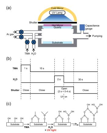
Fig. 1 (a) Schematic diagram of an ALD system equipped with a UV lamp. Cold mirror and hot mirror reflect UV radiation and visible/IR radiation, respectively. Note that the hot mirror prevents the substrate temperature from increasing. (b) UV-ALD sequence used for current study. (c) Sequential surface reactions to fabricate Al<sub>2</sub>O<sub>3</sub> thin films on a substrate using UV-ALD.
