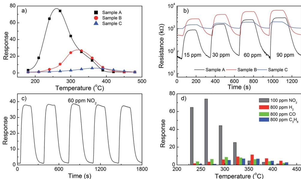
Fig. 4 The responses of ZnO architectures to 100 ppm NO<sub>2</sub> at operating temperature range of 180 °C to 480 °C (a); dynamic transient of resistances in response to NO<sub>2</sub> for ZnO architectures at 270 °C (b); response cycles of ZnO nanorods to 60 ppm at 300 °C (c); responses of ZnO nanorods for different gas (d).
