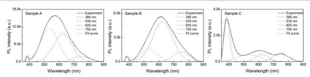
Fig. 3 PL spectra of hierarchical ZnO structures. The original spectra (black, solid lines) were resolved into several sub-bands (color, dash lines).
