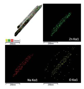
Fig. 2 STEM-mapping images of ZnO nanorods.
