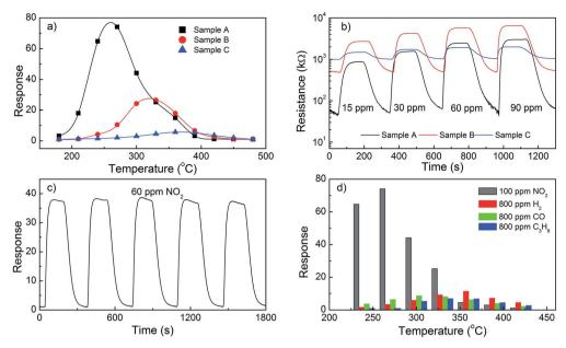
Fig. 4 The responses of ZnO architectures to 100 ppm  $NO_2$  at operating temperature range of 180 °C to 480 °C (a); dynamic transient of resistances in response to  $NO_2$  for ZnO architectures at 270 °C (b); response cycles of ZnO nanorods to 60 ppm at 300 °C (c); responses of ZnO nanorods for different gas (d).
