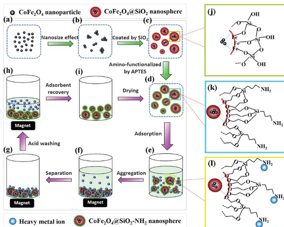
Fig. 1 Schematic illustration of the synthetic procedure of  $\text{CoFe}_2\text{O}_4@\text{SiO}_2\text{-NH}_2$  core-shell nanospheres (a–d, j and k) and the adsorption and regeneration process of heavy metals (d–i and l).
