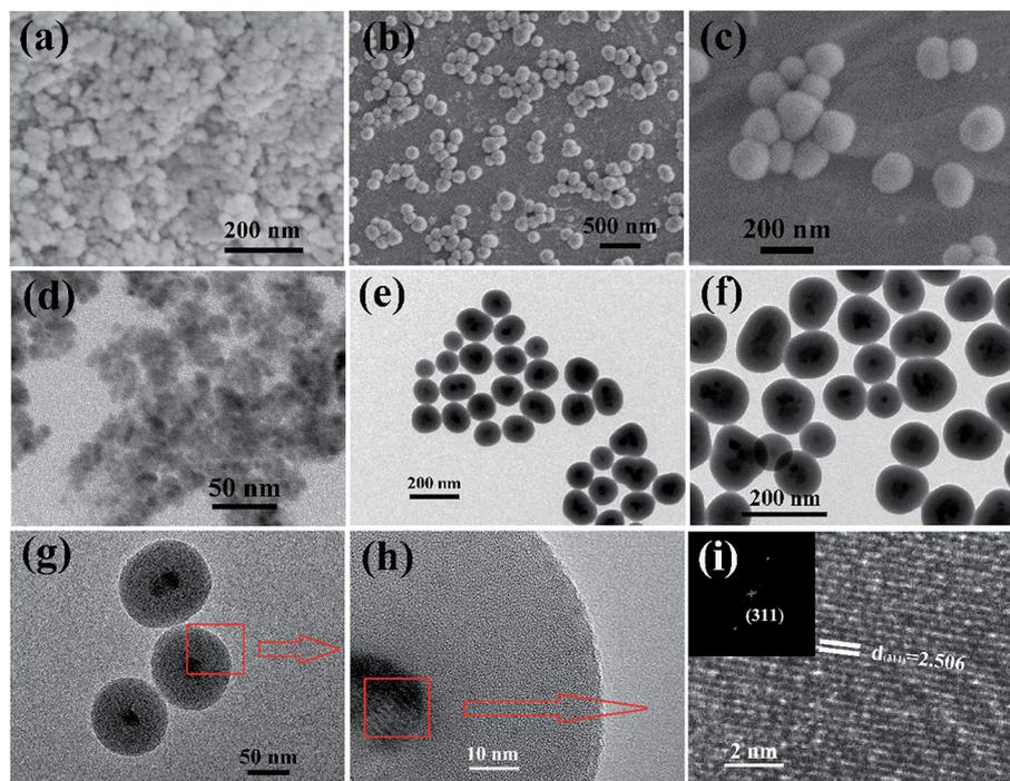
Fig. 2 SEM and TEM images of (a and d) CFO NPs, (b and e)  $\text{CFO}@\text{SiO}_2$ , and (c, f and g)  $\text{CFO}@\text{SiO}_2\text{-NH}_2$  nanospheres. (h and i) HRTEM images of  $\text{CFO}@\text{SiO}_2\text{-NH}_2$  nanospheres. (Inset of (i)) fast Fourier transform (FFT) pattern.
