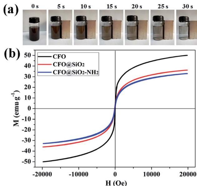
Fig. 3 (a) Dynamic pictures of magnetic separation process of CFO@SiO<sub>2</sub>-NH<sub>2</sub> and (b) room-temperature (300 K) magnetic hysteresis loops of CFO, CFO@SiO<sub>2</sub>, and CFO@SiO<sub>2</sub>-NH<sub>2</sub>.
