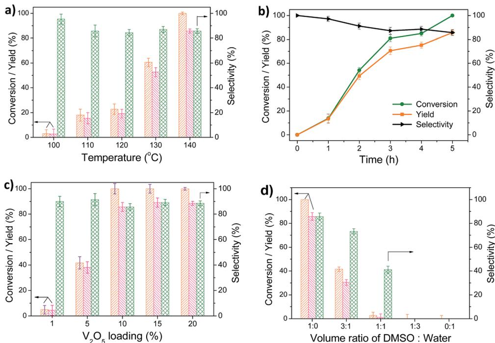
Fig. 4 The effects of different reaction conditions on the preparation of 2,5-DFF by the catalytic oxidation of 5-HMF using V-CP ((a) reaction temperature, (b) time, (c) V<sub>2</sub>O<sub>5</sub> content, and (d) DMSO/water volume ratio). If not specified, the default reaction conditions were as follows: 5-HMF, 63 mg; V-CP, 100 mg; V<sub>2</sub>O<sub>5</sub> content, 10%; solvent, DMSO; volume, 4 mL; O<sub>2</sub>, 40 mL min<sup>-1</sup>; temperature, 140 °C; and reaction time, 5 h.
