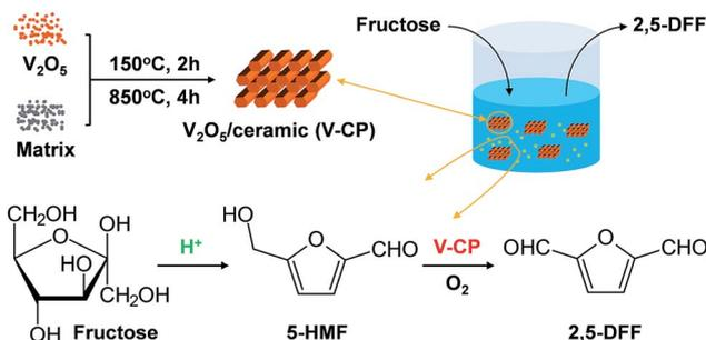
Scheme 1 Preparation of  $V_2O_5$ /ceramic catalyst and one-pot synthesis of 2,5-DFF from fructose.
