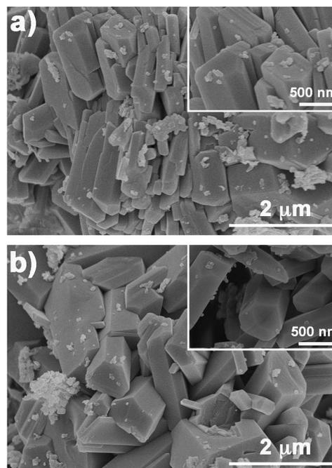
Fig. 1 SEM images of (a) ceramic matrix (CP) and (b) V<sub>2</sub>O<sub>5</sub>/ceramic catalyst.
