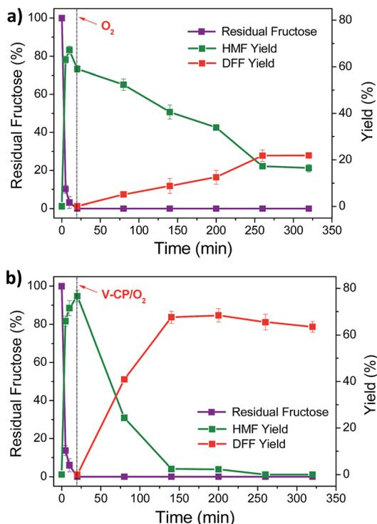
Fig. 6 Reaction curve of 2,5-DFF preparation by the one-pot  $V_2O_5$ /ceramic and diluted sulfuric acid co-catalysis method. (a) Adding V-CP at the beginning of the reaction together with acid and introducing oxygen after 20 min of reaction time. (b) Adding V-CP and oxygen after 20 min of reaction time. Reaction conditions: fructose, 90 mg; acid concentration, 0.05 M; V-CP, 100 mg; DMSO, 4 mL;  $O_2$ , 40 mL  $min^{-1}$ ; and reaction temperature, 140 °C.
