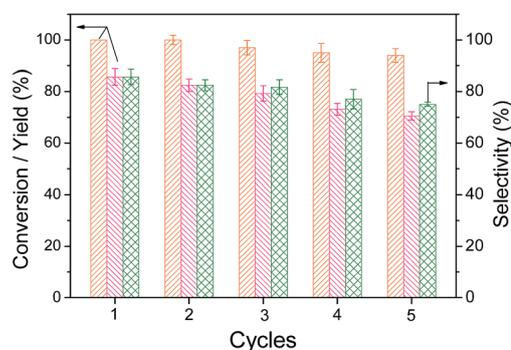
Fig. 5 Recycling and reuse of V-CP for 2,5-DFF production. Reaction conditions: 5-HMF, 63 mg; V-CP, 100 mg; V<sub>2</sub>O<sub>5</sub> content, 10%; DMSO, 4 mL; O<sub>2</sub>, 40 mL min<sup>-1</sup>; reaction temperature, 140 °C; and reaction time, 5 h.
