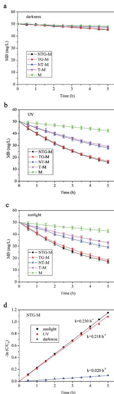
Fig. 7 Residual MB concentration treated by M, T-M, NT-M, TG-M and NTG-M in (a) darkness, (b) UV and (c) sunlight. (d) MB degradation kinetics for NTG-M in darkness, UV and sunlight. C<sub>0</sub> is the initial MB concentration (50 mg L<sup>-1</sup>), C is MB concentration at any time t.
