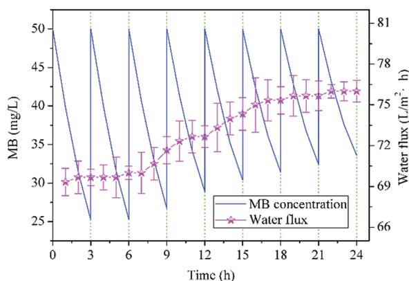
Fig. 9 Residual MB concentration treated by NTG-M in sunlight (the initial MB concentration was always  $50 \text{ mg L}^{-1}$ ) and pure water flux of NTG-M at 0.1 MPa at room temperature.
