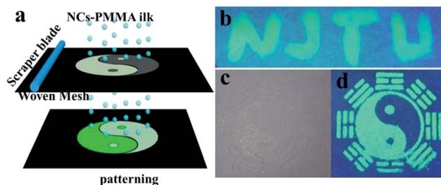
Fig. 6 (a) The schematic of patterning by screen printing. (b), (d) Images ( $\lambda_{\text{ex}} = 365 \text{ nm}$ ) and (c) (under daylight) of the patterning obtained using the mixture of CsPbBr<sub>3</sub> NC-PMMA.
