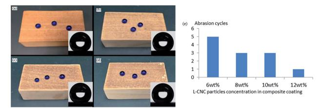
Fig. 6 Surface status of the coatings with L-CNC particles concentrations of (a) 6 wt%, (b) 8 wt%, (c) 10 wt%, and (d) 12 wt%; (e) bar charts of abrasion cycles of the coatings with different L-CNC particles concentration.
