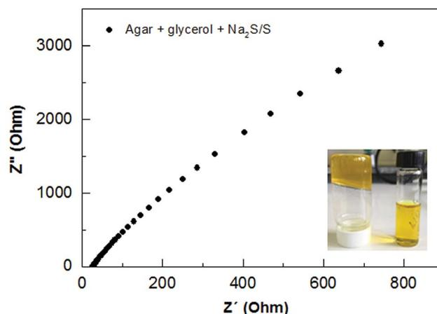
Fig. 4 Complex impedance plot for the agar-based gel electrolyte at room temperature.
