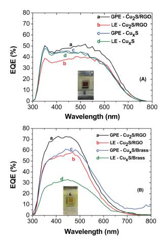
Fig. 7 IPCE curves of CuInS2 QDSSCs (A) CdS QDSSCs (B). The electrolyte and counter electrode used in both samples are shown in the inset
