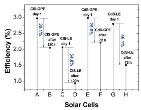
Fig. 8 Electrolyte stability for QDSSCs.
