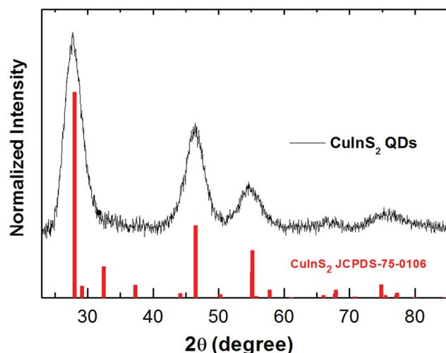
Fig. 3 X-ray diffraction pattern of CuInS<sub>2</sub> QDs and bulk pattern of chalcopyrite.
