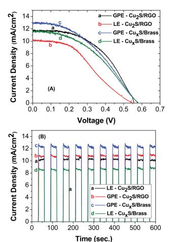
Fig. 6 Current-voltage characteristic (A) and photocurrent stability (B) of CdS QDSSCs. The electrolyte and counter electrode used in both experiments are shown in the inset.
