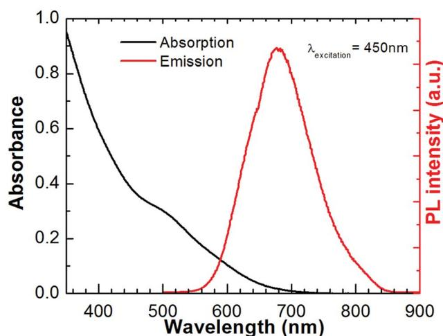
Fig. 1 Absorption and emission spectra for CuInS<sub>2</sub> QDs. Emission spectrum was recorded at 450 nm excitation wavelength in CHCl<sub>3</sub> solution.
