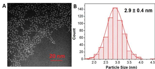
Fig. 2 (A) STEM image of CuInS<sub>2</sub> QDs showing the particles with pyramidal shape. (B) Size distribution of the particles with an average size of 2.9 nm.
