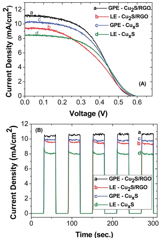
Fig. 5 Current–voltage characteristic (A) and photocurrent stability (B) of CuInS<sub>2</sub> QDSSCs. The electrolyte and counter electrode used in both experiments are shown in the inset.
