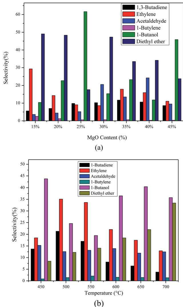
Fig. 9 The selectivity and products distribution of catalysts with different MgO contents (a), different calcination temperatures (b). Reaction temperature 673 K, WHSV 1.8 h<sup>-1</sup>.
