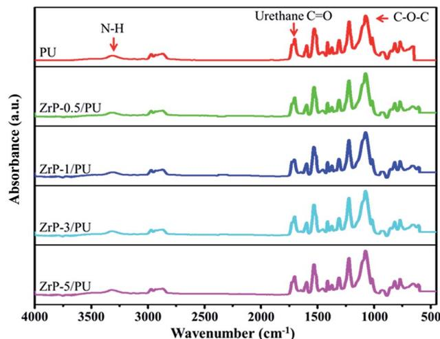
Fig. 3 FTIR spectra of PU and ZrP/PU films.
