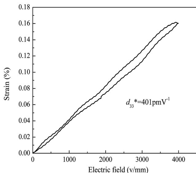
Fig. 4 Strain vs. unipolar electric field of the KNN47 single crystal at 1 Hz.
