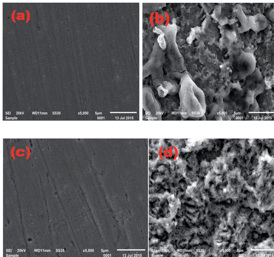
Fig. 6 SEM images of (a) plain MS surface, (b) MS in 0.5 M  $\text{H}_2\text{SO}_4$ , (c) MS in 0.5 M  $\text{H}_2\text{SO}_4 + 10^{-2}$  M EBTPPB, (d) MS in 0.5 M  $\text{H}_2\text{SO}_4 + 10^{-5}$  M EBTPPB, after 24 h exposure at the  $\times 5000$  magnification.
