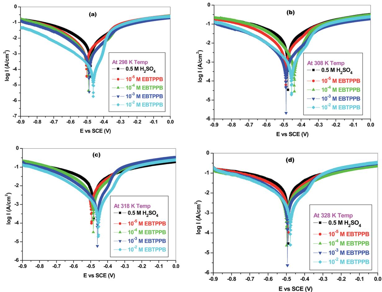
Fig. 2 Tafel polarisation curves for MS in 0.5 M H<sub>2</sub>SO<sub>4</sub> containing different concentrations of EBTTPB at temperatures (a) 298 K, (b) 308 K, (c) 318 K, and (d) 328 K.
