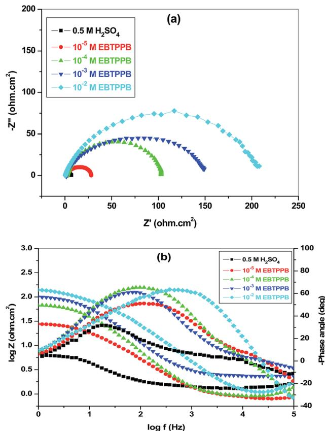
Fig. 3 Impedance plots for MS in 0.5 M H<sub>2</sub>SO<sub>4</sub> and in the presence of various concentrations of EBTPPB at 298 K. (a) Nyquist plot, and (b) Bode plot.
