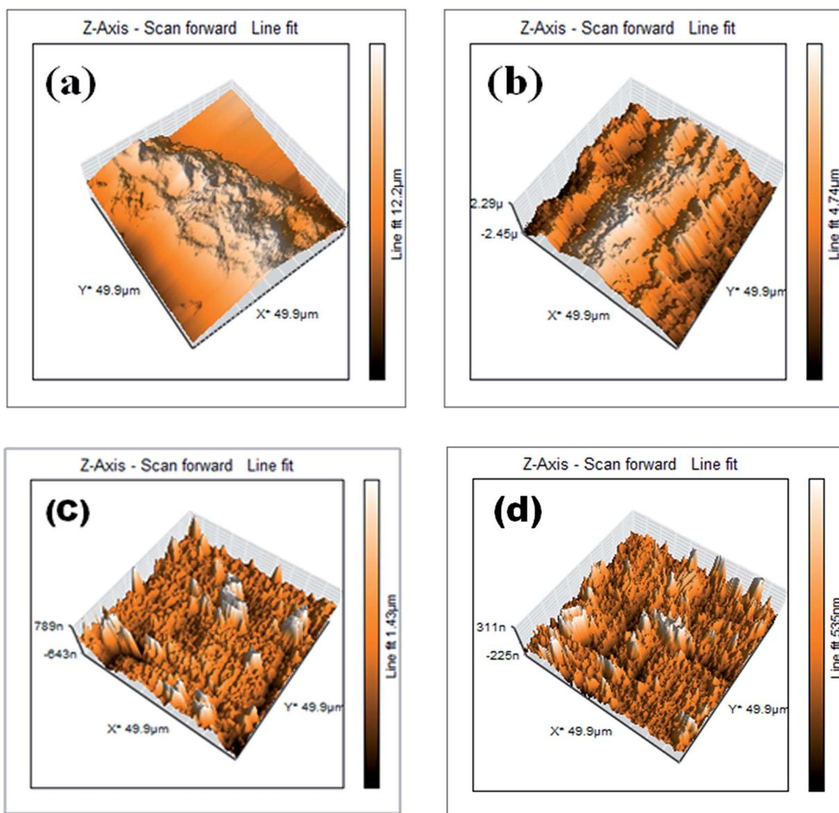
**Fig. 8** AFM images of (a) abraded MS surface, (b) MS in 0.5 M H<sub>2</sub>SO<sub>4</sub>, (c) MS in 0.5 M H<sub>2</sub>SO<sub>4</sub> + 10<sup>-2</sup> M EBTPPB (d) MS in 0.5 M H<sub>2</sub>SO<sub>4</sub> + 10<sup>-5</sup> M EBTPPB.
