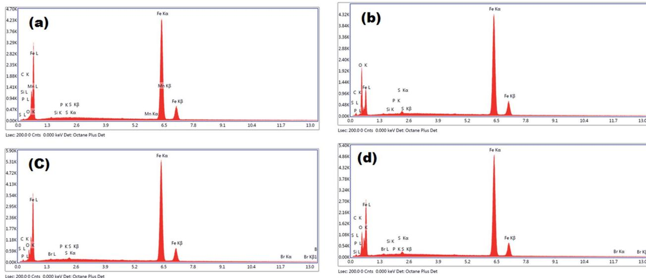
Fig. 7 EDXS spectra of (a) plain MS surface, (b) MS in 0.5 M  $\text{H}_2\text{SO}_4$ , (c) MS in 0.5 M  $\text{H}_2\text{SO}_4 + 10^{-2}$  M EBTPPB, (d) MS in 0.5 M  $\text{H}_2\text{SO}_4 + 10^{-5}$  M EBTPPB.
