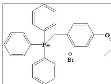
Fig. 1 The molecular structure of (4-ethoxybenzyl)-triphenylphosphonium bromide EBTPPB.
