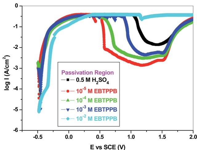
Fig. 5 Potentiostatic polarisation curves for MS in 0.5 M H<sub>2</sub>SO<sub>4</sub> containing different concentrations of EBTPPB at 298 K.
