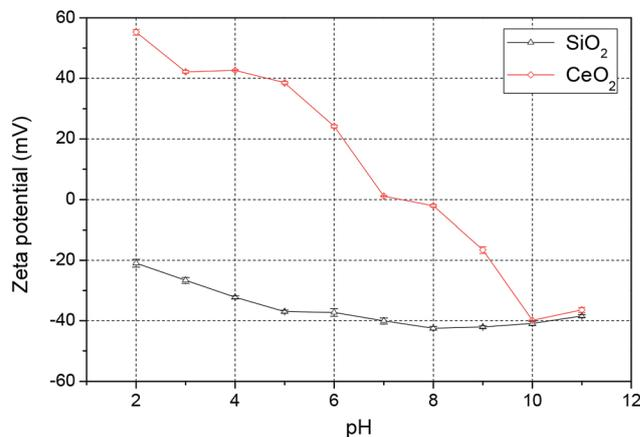
Fig. 2 Zeta potential of colloidal silica and ceria nanoparticles in DI water over the pH range 2–11.
