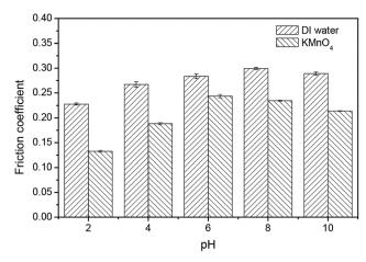
Fig. 10 The friction coefficients between the pad and the 6H-SiC substrate surface immersed in DI water and  $KMnO_4$  solution in pH range 2–10.
