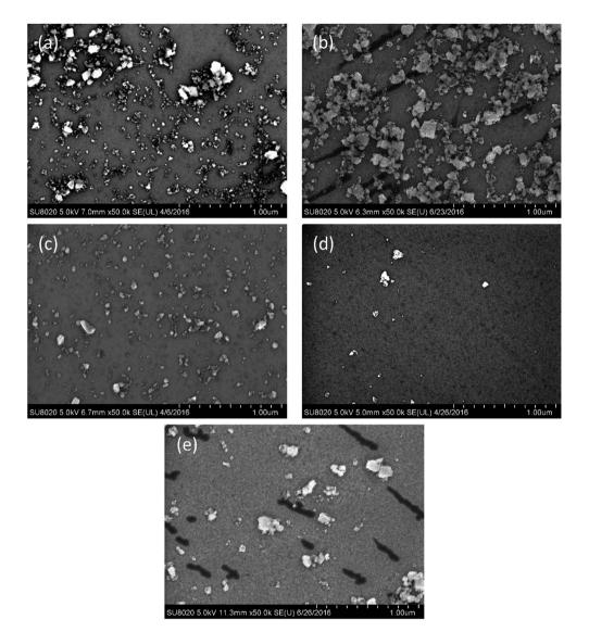
Fig. 7 The SEM images of the 6H-SiC substrate dipped in ceria + KMnO<sub>4</sub> based slurries at (a) pH 2, (b) pH 4, (c) pH 6, (d) pH 8 and (e) pH 10.
