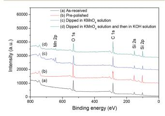
Fig. 16 XPS survey scans of the 6H-SiC surfaces: (a) as-received; (b) pre-polished; (c) dipped in  $KMnO_4$  solution; (d) dipped in  $KMnO_4$  solution and then in KOH solution.
