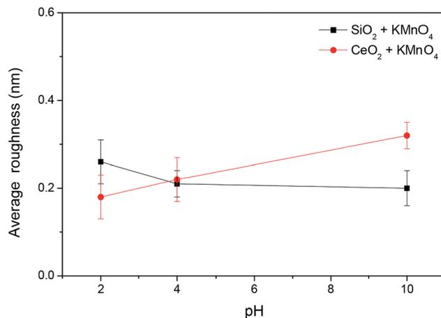
Fig. 15 The surface roughness of 6H-SiC substrates polished with silica-based slurries and ceria-based slurries in the presence of  $\text{KMnO}_4$  at pH 2, 4 and 10.
