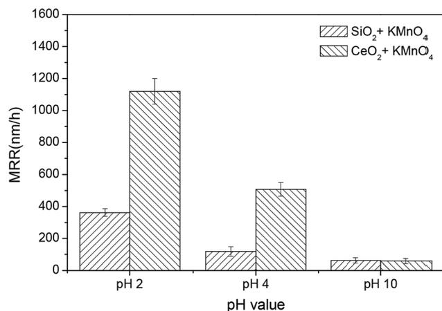
Fig. 13 The MRR of the 6H-SiC substrates polished with silica-based slurries and ceria-based slurries in the presence of KMnO<sub>4</sub> at pH 2, 4 and 10.
