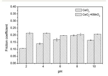
Fig. 12 The friction coefficients between the pad and the 6H-SiC substrate surface immersed in the ceria based slurries in the absence and presence of  $KMnO_4$  in a pH range of 2–10.
