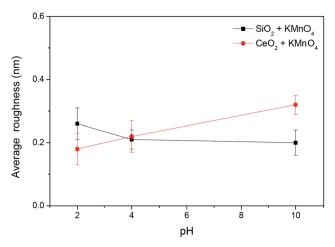
Fig. 15 The surface roughness of 6H-SiC substrates polished with silica-based slurries and ceria-based slurries in the presence of KMnO<sub>4</sub> at pH 2, 4 and 10.
