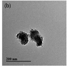
Fig. 1 The TEM images of the abrasive nanoparticles: (a) silica; (b) ceria.
