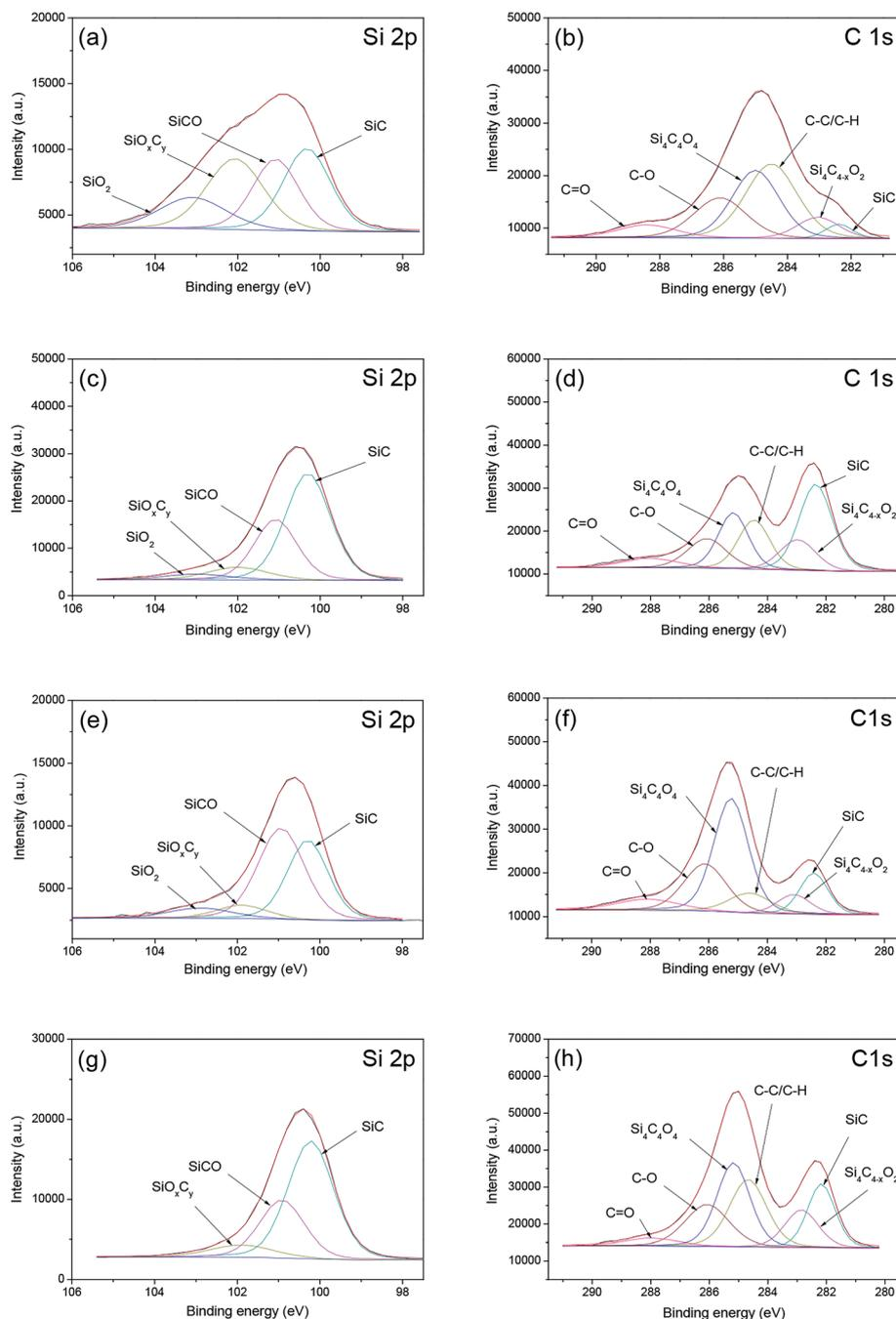
Fig. 17 Si 2p and C 1s spectra of the 6H-SiC surfaces: (a and b) as-received; (c and d) pre-polished; (e and f) dipped in  $\text{KMnO}_4$  solution; (g and h) dipped in  $\text{KMnO}_4$  solution and then in  $\text{KOH}$  solution.
