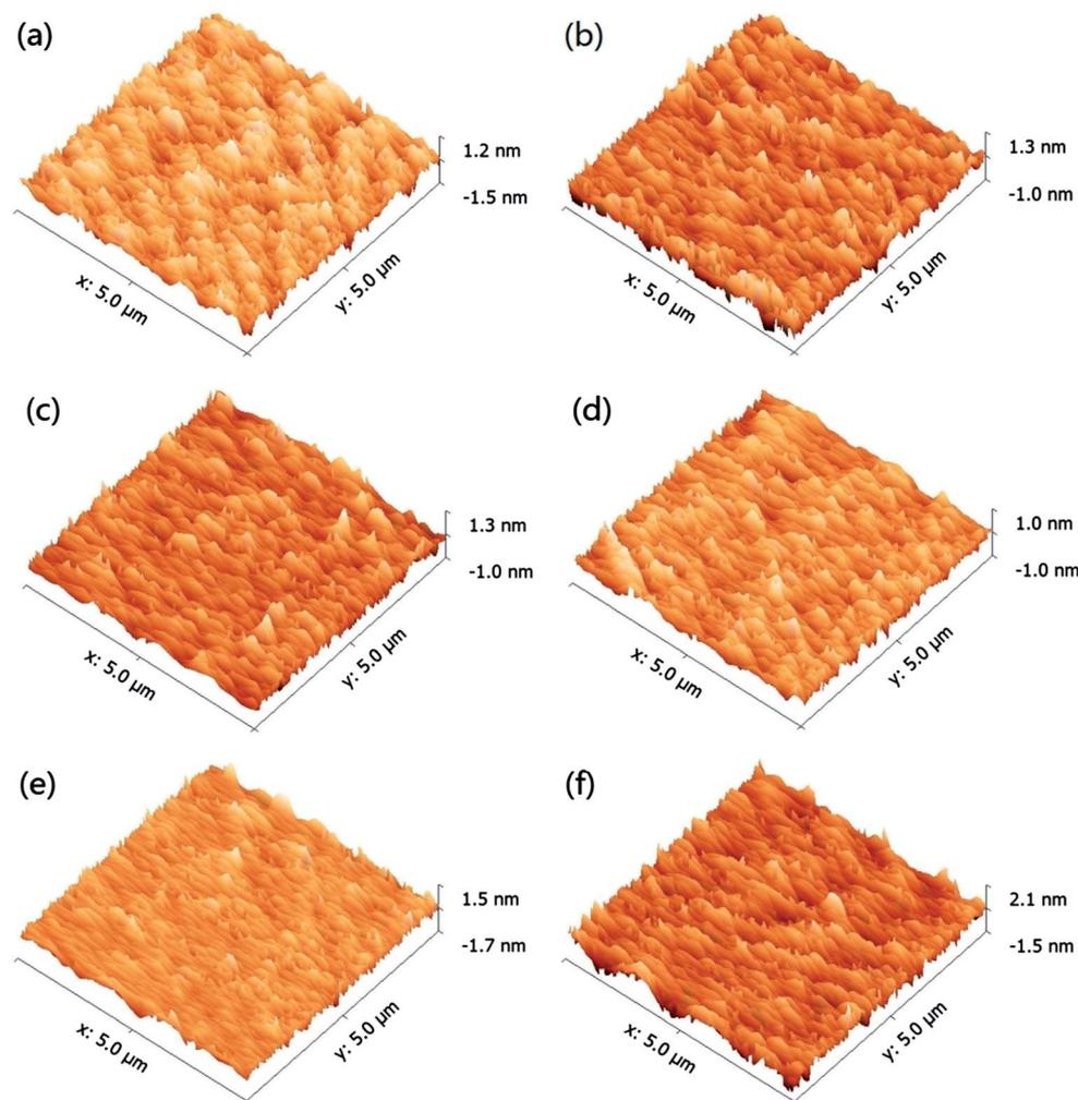
Fig. 14 AFM images of the 6H-SiC surfaces polished with silica + KMnO<sub>4</sub> based slurries at (a) pH 2, (b) pH 4, (c) pH 10 and with ceria + KMnO<sub>4</sub> based slurries at (d) pH 2, (e) pH 4, (f) pH 10.
