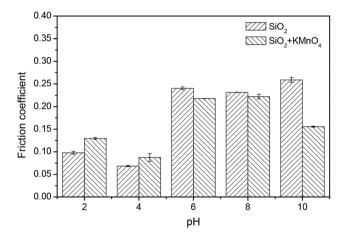
Fig. 11 The friction coefficients between the pad and the 6H-SiC substrate surface immersed in the silica based slurries in the absence and presence of  $KMnO_4$  in a pH range of 2–10.
