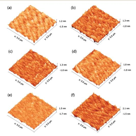
Fig. 14 AFM images of the 6H-SiC surfaces polished with silica +  $KMnO_4$  based slurries at (a) pH 2, (b) pH 4, (c) pH 10 and with ceria +  $KMnO_4$  based slurries at (d) pH 2, (e) pH 4, (f) pH 10.
