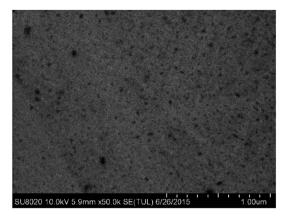
Fig. 3 The SEM image of the as-received 6H-SiC substrate.
