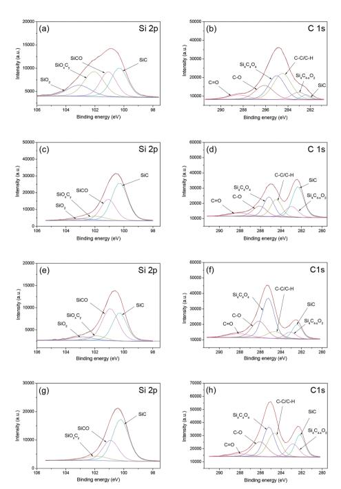
Fig. 17 Si 2p and C 1s spectra of the 6H-SiC surfaces: (a and b) as-received; (c and d) pre-polished; (e and f) dipped in  $KMnO_4$  solution; (g and h) dipped in  $KMnO_4$  solution and then in KOH solution.
