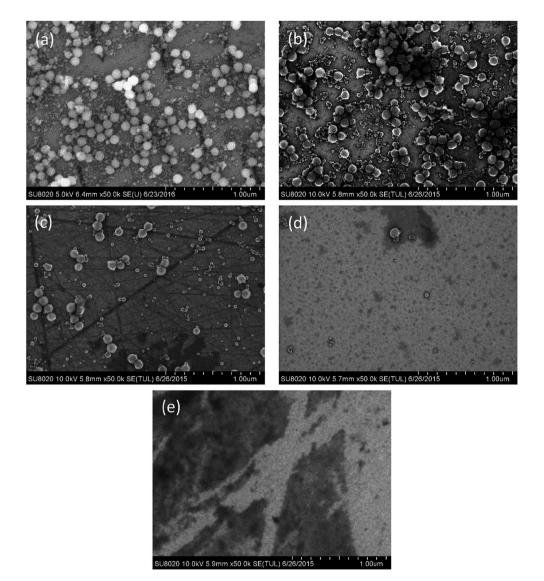
The SEM images of the 6H-SiC substrate dipped in silica + KMnO<sub>4</sub> based slurries at (a) pH 2, (b) pH 4, (c) pH 6, (d) pH 8 and (e) pH 10.
