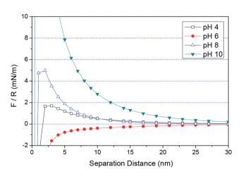
Fig. 9 The normalized forces between the surfaces of 6H-SiC and ceria particles as a function of separation distance at different pH values. The surface potentials of the SiC plate and ceria particles are 30 and 43 mV at pH 4, -56 and 24 mV at pH 6, -96 and -2 mV at pH 8, -125 and -40 mV at pH 10, respectively. The Hamaker constant is 8.5  $\times$   $10^{-20}$  J and the background electrolyte is 1 mM KNO3.
