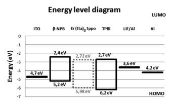
Fig. 9 Energy level diagram of device with the structure: ITO/β-NPB (30 nm)/[Er(tta)<sub>3</sub>(tppo)] (40 nm)/TPBi (30 nm)/LiF (0.1 nm)/Al (100 nm).
