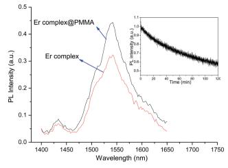
Fig. 7 NIR emission spectra of the complex in pure form and PMMAdoped sample, under excitation ( $\lambda_{max} = 380$  nm). Inset: photostability curve of the complex.
