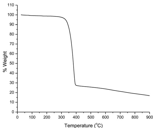
Fig. 1 TGA curve of the complex.
