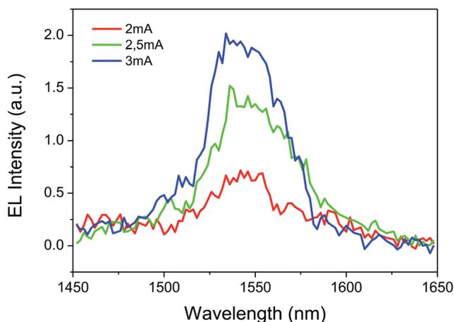
Fig. 10 Electroluminescence spectra of the complex.
