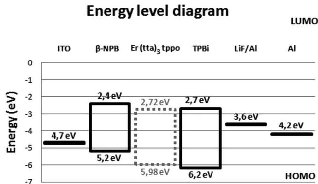
Fig. 9 Energy level diagram of device with the structure: ITO/ $\beta$ -NPB (30 nm)/[Er(tta)<sub>3</sub>(tppo)] (40 nm)/TPBi (30 nm)/LiF (0.1 nm)/Al (100 nm).
