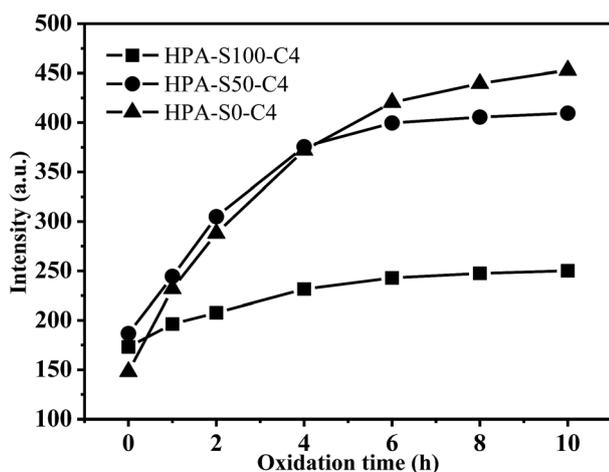
Fig. 9 Influence of oxidation time on fluorescence emission intensity of HPA-C4s (polymer concentration is 5 mg mL<sup>-1</sup>; excitation wavelength is 370 nm; slit widths of excitation and emission are set to be 10 nm and 10 nm, respectively).
