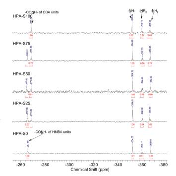
Fig. 2 <sup>15</sup>N NMR spectra of HPAs.
