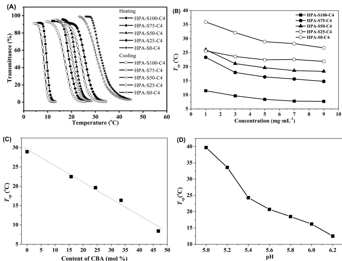
Fig. 6 (A) Typical temperature-dependent light transmittance of the aqueous solutions of HPA-C4s (concentration of polymer is 5  $\text{mg mL}^{-1}$ ); (B) effect of the concentration of HPA-C4s in de-ionized water on the  $T_{cp}$ ; (C) effect of the CBA content in HPA-C4s on the  $T_{cp}$  (concentration of polymer is 5  $\text{mg mL}^{-1}$ ) and (D) effect of pH on the  $T_{cp}$  (HPA-S100-C4 as the representative).
