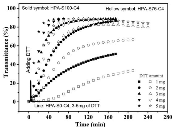
Fig. 7 Time-dependent transmittance of the aqueous solutions of HPA-S100–C4, HPA-S75–C4 and HPA-S0–C4 upon the addition of different amount of DTT (polymer concentration is 5 mg mL<sup>-1</sup>, 37 °C).
