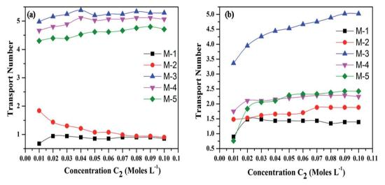
Fig. 5 Effect of concentration on transport numbers for (a) alkali (Na<sup>+</sup>) and (b) alkaline earth (Ba<sup>2+</sup>) metal ions.
