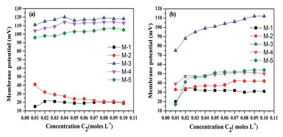
Fig. 4 Effect of concentration on membrane potential values for (a) alkali (Na<sup>+</sup>) and (b) alkaline earth (Ba<sup>2+</sup>) metal ions.
