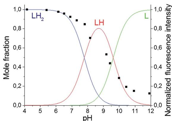
Fig. 2 Fluorescence emission pH titration curve of compound 5 (10  $\mu\text{M}$ ,  $\lambda_{\text{ex}} = 472 \text{ nm}$ ,  $\lambda_{\text{em}} = 552 \text{ nm}$ ) in water (black  $\blacksquare$ ) and mole fraction distribution diagram for the various protonated species of this ligand (solid lines).
