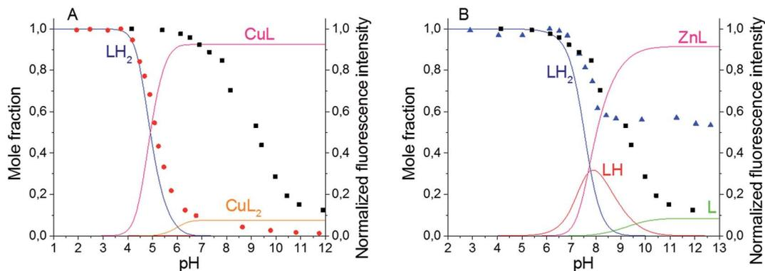
Fig. 3 Fluorescence emission pH titration curves of compound 5 (10  $\mu$ M,  $\lambda_{\text{ex}} = 472$  nm,  $\lambda_{\text{em}} = 552$  nm) in water in the absence (black  $\blacksquare$ ) or presence of 1 equivalent of metal ion, (A) Cu(II) (red  $\bullet$ ) and (B) Zn(II) (blue  $\blacktriangle$ ), and mole fraction distribution diagrams for the various species of this ligand under these conditions (solid lines).
