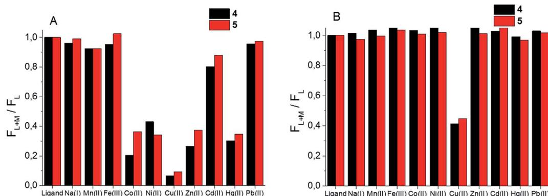
Fig. 5 Fluorescence response of ligands 4 (10  $\mu$ M,  $\lambda_{\text{ex}} = 472$  nm,  $\lambda_{\text{em}} = 576$  nm) and 5 (10  $\mu$ M,  $\lambda_{\text{ex}} = 472$  nm,  $\lambda_{\text{em}} = 552$  nm) to an excess (4 equivalents) of selected metal ions in an aqueous sodium cacodylate buffer solution (0.05 M) at (A) pH 7.4 and (B) pH 5.  $F_L$  and  $F_{L+M}$  denote the normalized fluorescence intensity of the free ligand and the ligand in the presence of the metal ion, respectively.
