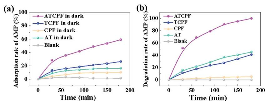
Fig. 5 (a) The adsorption of AMP in dark condition within the presence of ATCPF, TCPF, CPF, AT nanoparticles and blank polypropylene film; (b) the degradation of AMP (20 mg L<sup>-1</sup>, 40 mL) during simulated solar irradiation in the presence of ATCPF, TCPF, CPF, Ag<sub>2</sub>O/TiO<sub>2</sub> nanocomposites (AT) and blank polypropylene film.
