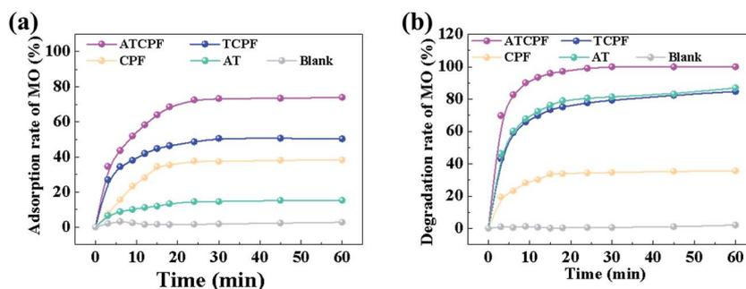
Fig. 6 (a) The adsorption of MO (10 mg L<sup>-1</sup>, 40 mL) in dark condition within the presence of ATCPF, TCPF, CPF, AT and blank film polypropylene. (b) The degradation of MO (10 mg L<sup>-1</sup>, 40 mL) during simulated solar irradiation in the presence of ATCPF, TCPF, CPF, AT and blank polypropylene film.
