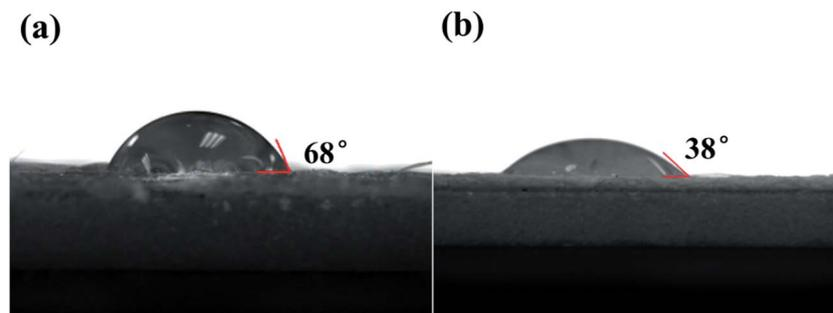
Fig. 4 Contact angle characterization of (a) blank film and (b) ATCPF.
