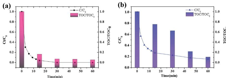
Fig. 7 Concentration change and TOC analysis of (a) ATCPF, (b) TCPF during photocatalytic degradation of MO ( $C_{0, \text{MO}} = 10 \text{ mg L}^{-1}$ ;  $V = 40 \text{ mL}$ ;  $M = 0.075 \text{ g}$ ;  $N = 70 \text{ rpm}$ ; UV;  $t = 6 \text{ h}$ ).
