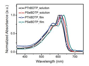
Fig. 2 Absorption spectra for PThBDTP<sub>i</sub> and PSeBDTP<sub>i</sub> in solution and as films
