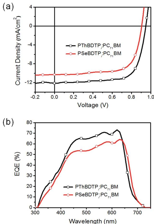
Fig. 4  $J$ - $V$  curves (a) and EQE spectra (b) for polymer:PC<sub>71</sub>BM solar cells.
