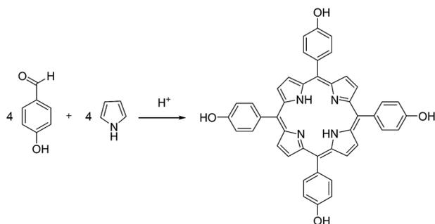
Scheme 1 Schematic representation of the synthesis of THPP.
