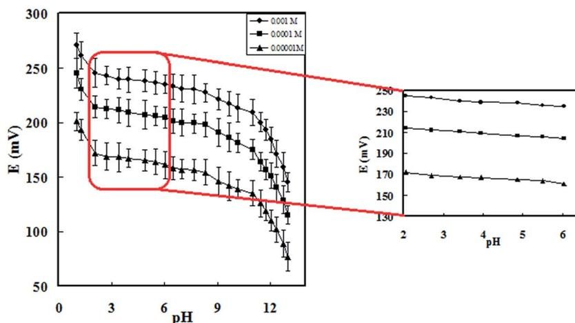
Fig. 3 Effect of pH on the response of the modified electrode ( $\mu = 0.10$ ; NaCl).
