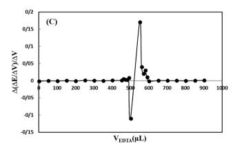
Fig. 5 (A) Potentiometric titration curve of 50.0 mL of  $5.0 \times 10^{-4}$  mol L<sup>-1</sup> Cu(NO<sub>3</sub>)<sub>2</sub> solution with  $5.0 \times 10^{-2}$  mol L<sup>-1</sup> EDTA, using IIP based CPE as indicator electrode, (B) its first and (C) second derivatives curves (pH = 4.5,  $\mu$  = 0.10; NaCl).
