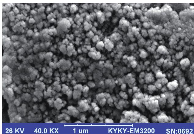
Fig. 2 SEM image of the prepared Cu-IIP particles.
