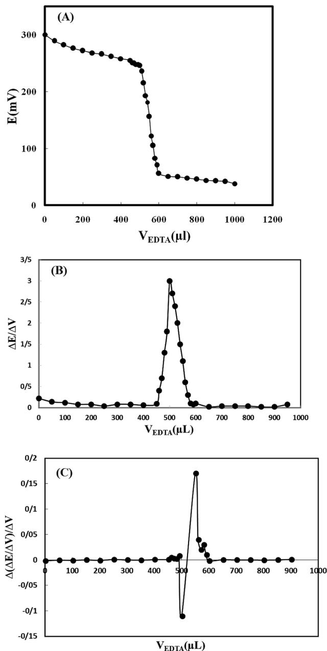
Fig. 5 (A) Potentiometric titration curve of 50.0 mL of  $5.0 \times 10^{-4}$  mol L<sup>-1</sup> Cu(NO<sub>3</sub>)<sub>2</sub> solution with  $5.0 \times 10^{-2}$  mol L<sup>-1</sup> EDTA, using IIP based CPE as indicator electrode, (B) its first and (C) second derivatives curves (pH = 4.5,  $\mu = 0.10$ ; NaCl).
