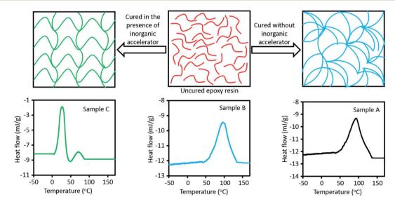
Fig. 4 Comparison of arrangement of epoxy structure with and without inorganic accelerator (top), and heat flow *versus* temperature obtained for the various samples at heating rate of 10  $^{\circ}$ C min $^{-1}$  (bottom).
