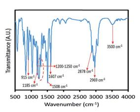
Fig. 3 FT-IR spectrum of synthesized vanillin-based epoxy resin.
