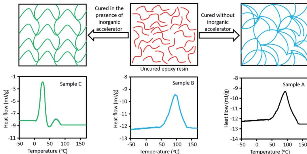
Fig. 4 Comparison of arrangement of epoxy structure with and without inorganic accelerator (top), and heat flow versus temperature obtained for the various samples at heating rate of  $10\text{ }^\circ\text{C min}^{-1}$  (bottom).
