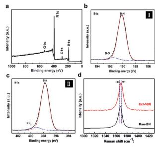
Fig. 2 A comparison of the properties of Exf-hBN and Raw-BN. (a) XPS survey scan of Exf-hBN. (b) The high-resolution XPS B 1s spectra of Exf-hBN. (c) High-resolution XPS N 1s spectra of Exf-hBN. (d) The Raman spectra of Exf-hBN and Raw-BN.
