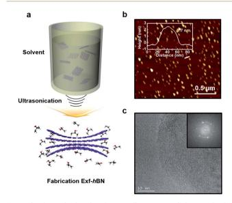
Fig. 1 A schematic showing the overall process and characterization of Exf-hBN. (a) A schematic of the strategy used to prepare Exf-hBN. (b) An AFM image of Exf-hBN on a mica substrate. (c) The HRTEM image and fringe patterns of Exf-hBN.
