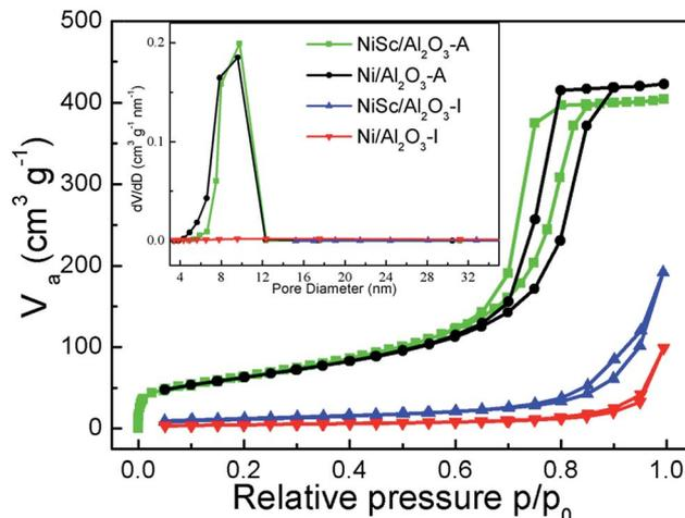
Fig. 3 Nitrogen adsorption-desorption isotherms; (inset) pore size distributions of various catalysts.
