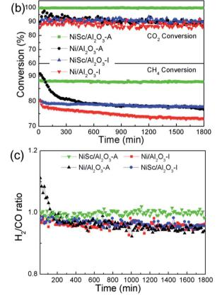
Fig. 6 (a)  $CH_4$  and  $CO_2$  conversions over various catalysts at different temperatures; (b) catalytic stability test and (c)  $H_2/CO$  ratios of various catalysts for methane dry reforming at 750 °C for 1800 min. (Catalytic conditions:  $CH_4$ :  $CO_2 = 1$ : 1, 15 mL min<sup>-1</sup> per reactor; 150 mg of catalysts.)
