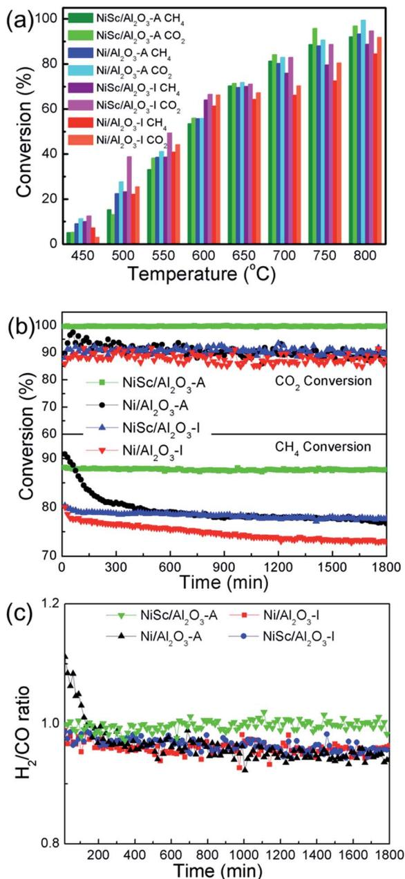
Fig. 6 (a) CH<sub>4</sub> and CO<sub>2</sub> conversions over various catalysts at different temperatures; (b) catalytic stability test and (c) H<sub>2</sub>/CO ratios of various catalysts for methane dry reforming at 750 °C for 1800 min. (Catalytic conditions: CH<sub>4</sub> : CO<sub>2</sub> = 1 : 1, 15 mL min<sup>-1</sup> per reactor; 150 mg of catalysts.)
