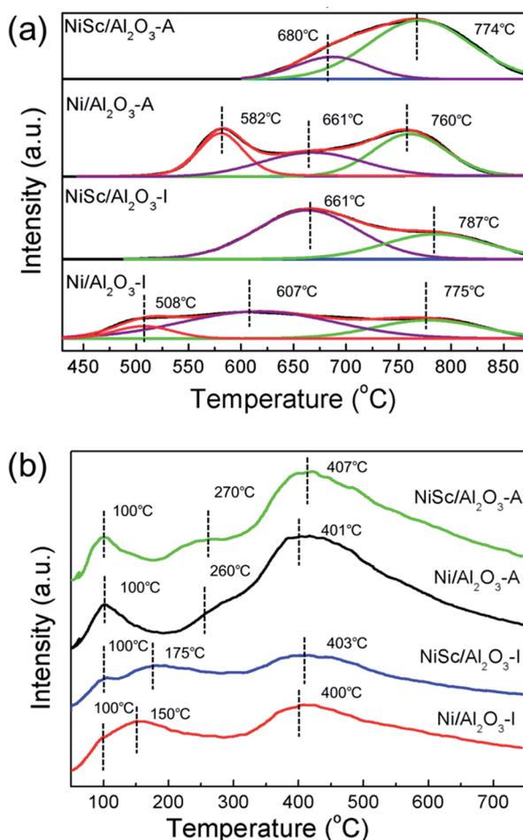
Fig. 4 (a) H<sub>2</sub>-TPR profiles and (b) CO<sub>2</sub>-TPD profiles of various catalysts after reduction.
