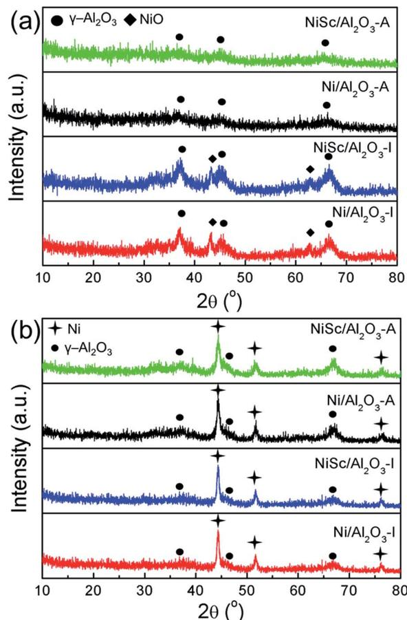
Fig. 2 XRD patterns for (a) the various catalysts after calcination; and (b) after reduction.
