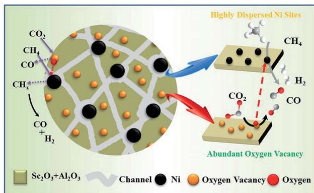
Fig. 9 Mechanism of methane dry reforming over NiSc/Al<sub>2</sub>O<sub>3</sub>-A catalyst.
