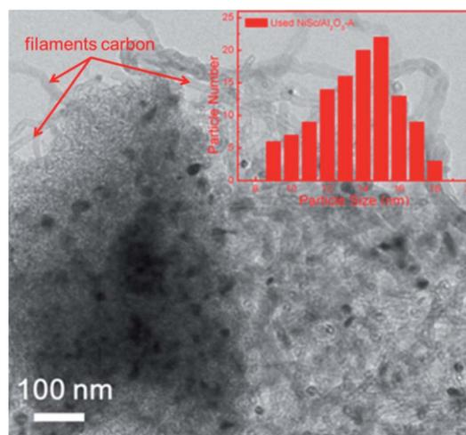
Fig. 8 TEM image and nickel particle size distributions of NiSc/Al<sub>2</sub>O<sub>3</sub>-A catalyst after 1800 min tested.
