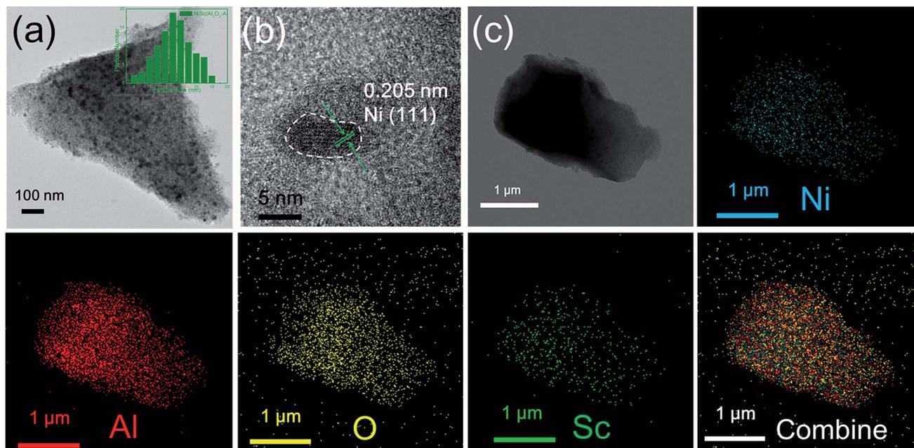
Fig. 1 (a) TEM image (inset: the size distributions of Ni NPs); (b) HRTEM image and (c) EDX mapping of the fresh NiSc/Al<sub>2</sub>O<sub>3</sub>-A catalyst.
