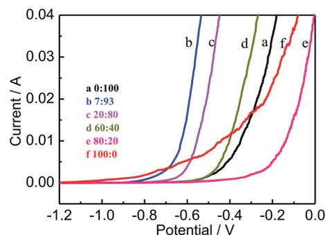
Fig. 1 LSV curves of AZ31B Mg alloys in different volume ratio of  $\text{MgSO}_4 : \text{Mg}(\text{NO}_3)_2$ ; 0 : 100 (a), 7 : 93 (b), 20 : 80 (c), 60 : 40 (d), 80 : 20 (e) and 100 : 0 (f).
