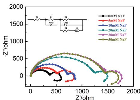
**Fig. 3** EIS plots of AZ31B Mg alloy in composite electrolyte solution (MgSO<sub>4</sub> : Mg(NO<sub>3</sub>)<sub>2</sub> = 7 : 93) with different concentrations of NaF.
