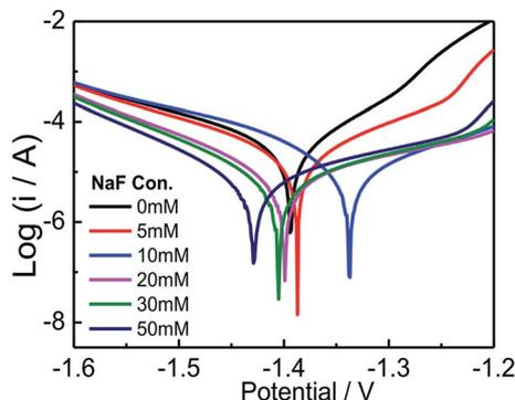
Fig. 2 Tafel curves of AZ31B alloy in composite solution (MgSO<sub>4</sub> : Mg(NO<sub>3</sub>)<sub>2</sub> = 7 : 93) with different concentrations of NaF.
