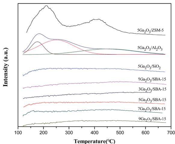
Fig. 5 NH<sub>3</sub>-TPD profiles of the different catalysts.
