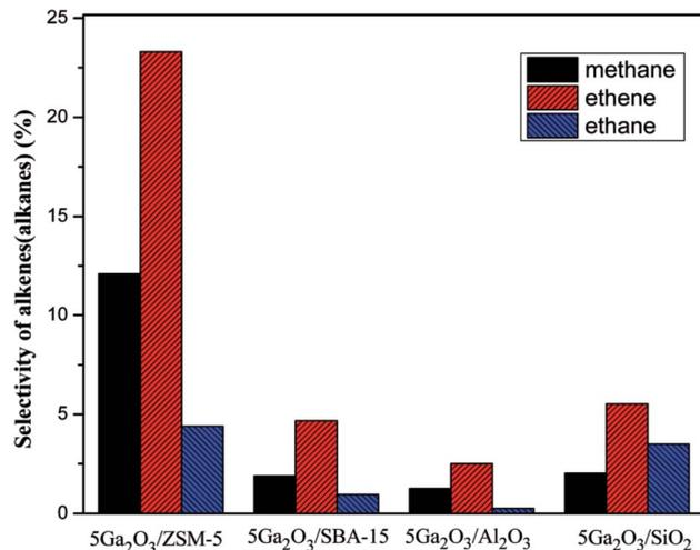
Fig. 9 Selectivities to alkanes (alkenes) over the different catalysts in the initial 30 min reaction: (reaction conditions:  $T = 620\text{ }^{\circ}\text{C}$ ;  $\text{C}_3\text{H}_8$  : Ar (molar ratio) = 1 : 19;  $\text{WHSV} = 0.6\text{ h}^{-1}$ ;  $m_{\text{cat.}} = 0.2\text{ g}$ ).
