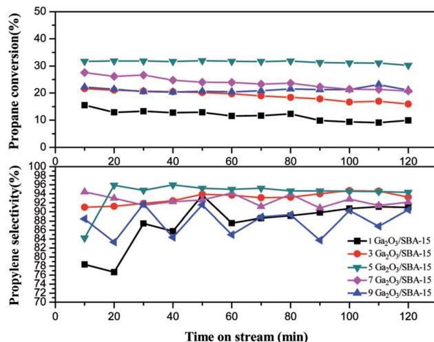
Fig. 10 The effect of  $\text{Ga}_2\text{O}_3$  content of the catalysts on the catalytic performance in propane dehydrogenation (reaction conditions:  $T = 620\text{ }^{\circ}\text{C}$ ;  $\text{C}_3\text{H}_8$  : Ar (molar ratio) = 1 : 19;  $\text{WHSV} = 0.6\text{ h}^{-1}$ ;  $m_{\text{cat.}} = 0.2\text{ g}$ ).
