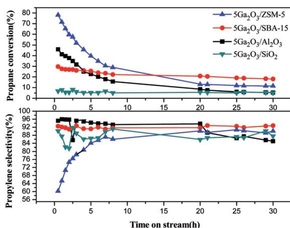
Fig. 8 Propane conversion and propylene selectivity of the different catalysts as a function of time (reaction conditions:  $T = 620\text{ }^{\circ}\text{C}$ ;  $\text{C}_3\text{H}_8 : \text{Ar}$  (molar ratio) = 1 : 19;  $\text{WHSV} = 0.6\text{ h}^{-1}$ ;  $m_{\text{cat}} = 0.2\text{ g}$ ).
