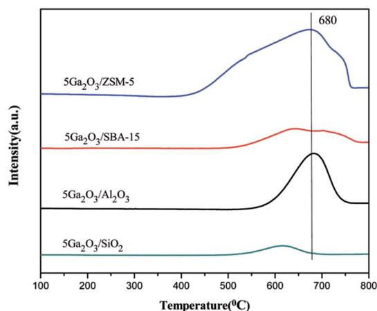
Fig. 12 TPO profiles of the spent catalysts.
