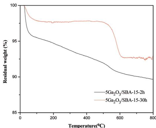
Fig. 13 TG profiles of the spent  $5\text{Ga}_2\text{O}_3/\text{SBA-15}$  catalysts.
