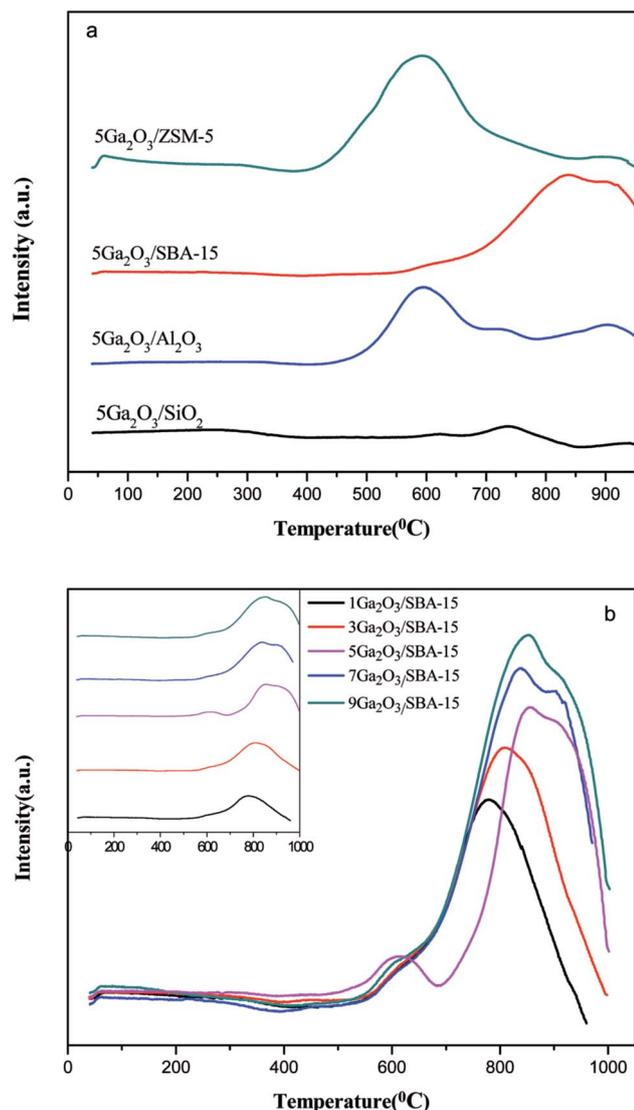
Fig. 6 H<sub>2</sub>-TPR profiles of the different catalysts.
