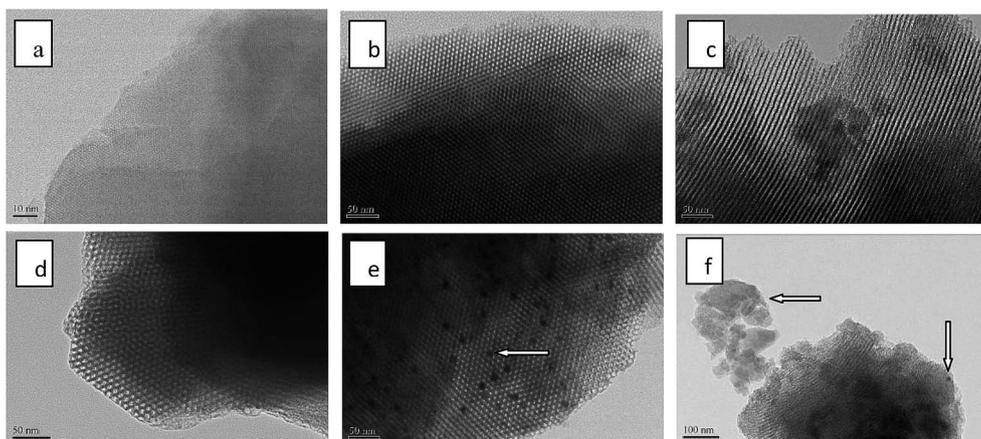
Fig. 4 TEM micrographs of (a) 5Ga<sub>2</sub>O<sub>3</sub>/ZSM-5; (b) 1Ga<sub>2</sub>O<sub>3</sub>/SBA-15; (c) 3Ga<sub>2</sub>O<sub>3</sub>/SBA-15; (d) 5Ga<sub>2</sub>O<sub>3</sub>/SBA-15; (e) 7Ga<sub>2</sub>O<sub>3</sub>/SBA-15; (f) 9Ga<sub>2</sub>O<sub>3</sub>/SBA-15.
