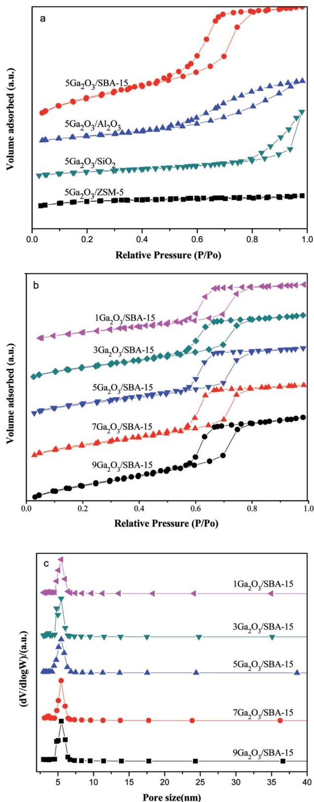
Fig. 1 (a) and (b) Low temperature  $\text{N}_2$  adsorption–desorption isotherms of  $x\text{Ga}_2\text{O}_3/\text{SBA-15}$ ,  $5\text{Ga}_2\text{O}_3/\text{Al}_2\text{O}_3$ ,  $5\text{Ga}_2\text{O}_3/\text{SiO}_2$ ,  $5\text{Ga}_2\text{O}_3/\text{ZSM-5}$  catalysts and (c) the corresponding pore size distributions of  $x\text{Ga}_2\text{O}_3/\text{SBA-15}$  catalysts.
