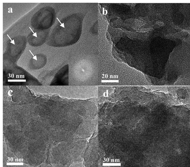
Fig. 3 TEM images of Y-NA samples obtained at different crystallization times (a) 4 h, (b) 8 h, (c) 12 h and (d) 16 h. Inset of (a) electron diffraction pattern.
