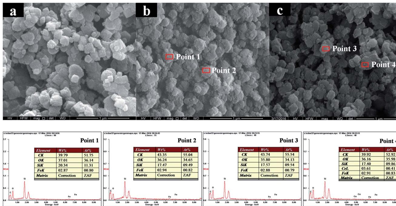
Fig. 3 SEM images and EDX analysis for pure H-beta (a); Fe/beta (b); Mo<sub>0.2</sub>-Fe/beta (c).
