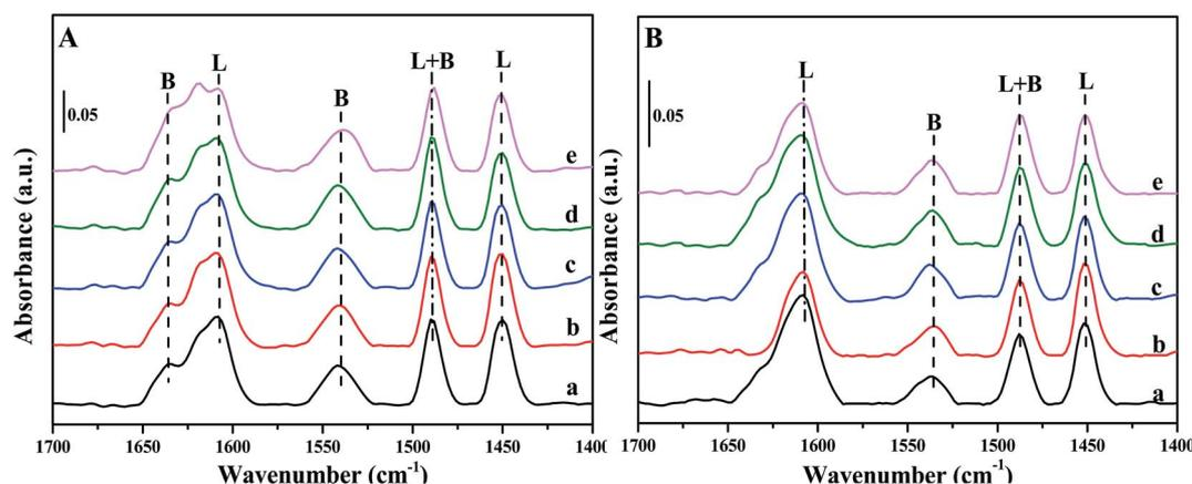
Fig. 6 FT-IR spectra of pyridine adsorbed on Fe/beta (a);  $\text{Mo}_{0.1}$ -Fe/beta (b);  $\text{Mo}_{0.2}$ -Fe/beta (c);  $\text{Mo}_{0.5}$ -Fe/beta (d);  $\text{Mo}_1$ -Fe/beta (e) after degassing at 200 °C (A) and 350 °C (B).
