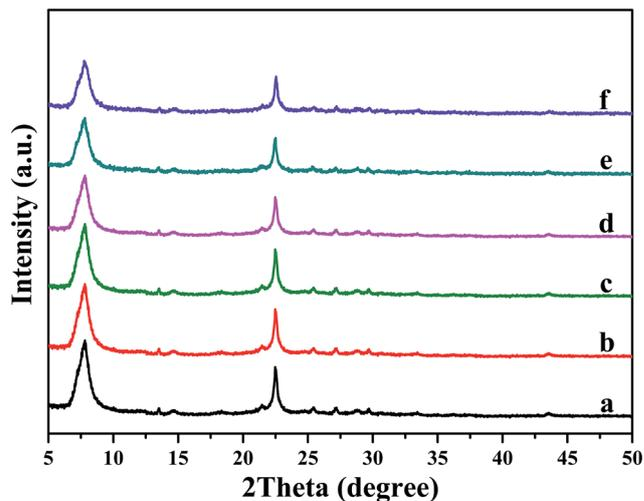
Fig. 2 XRD patterns of pure H-beta (a);  $\text{Fe}/\beta$  (b);  $\text{Mo}_{0.1}\text{-Fe}/\beta$  (c);  $\text{Mo}_{0.2}\text{-Fe}/\beta$  (d);  $\text{Mo}_{0.5}\text{-Fe}/\beta$  (e);  $\text{Mo}_1\text{-Fe}/\beta$  (f).
