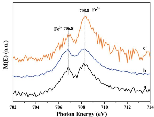
Fig. 9 XANES spectra of the catalysts: Fe/beta (a),  $\text{Mo}_{0.2}$ -Fe/beta (b),  $\text{Mo}_{0.5}$ -Fe/beta (c).
