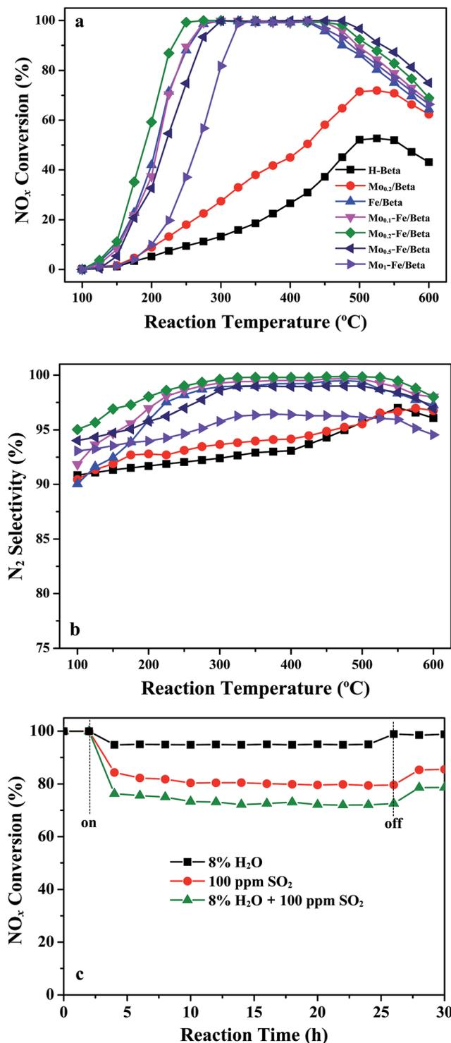
Fig. 1  $\text{NO}_x$  conversion (a) and  $\text{N}_2$  selectivity (b) as a function of reaction temperature over pure H-beta, Mo/beta, Fe/beta and  $\text{Mo}_x\text{-Fe/beta}$  catalysts with variable Mo loading amounts in the temperature range of 100–600 °C. (c)  $\text{NO}_x$  conversion in the presence of  $\text{H}_2\text{O}$  and/or  $\text{SO}_2$  over  $\text{Mo}_{0.2}\text{-Fe/beta}$  catalyst at 300 °C.
