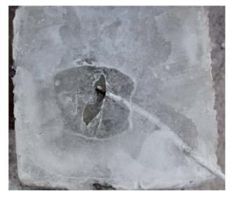
Fig. 8 Ice after microwave irradiation.
