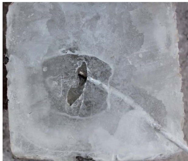
Fig. 8 Ice after microwave irradiation.
