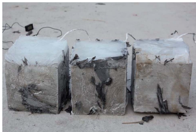
Fig. 7 Specimens covered with ice layer.
