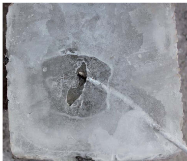
Fig. 8 Ice after microwave irradiation.
