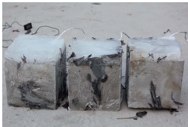
Fig. 7 Specimens covered with ice layer.
