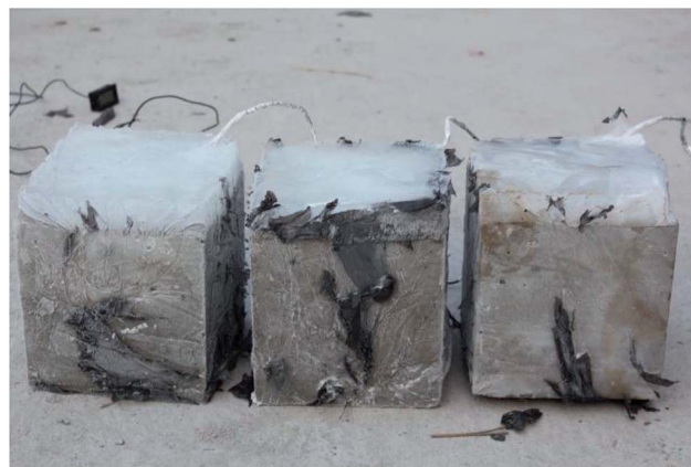
Fig. 7 Specimens covered with ice layer.
