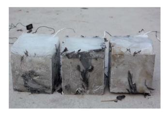
Fig. 7 Specimens covered with ice layer.
