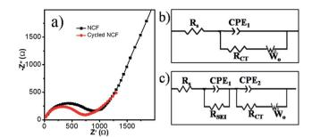
Fig. 6 Nyquist plots of the Na/NCF half cells in different states (a), the corresponding equivalent circuits for an as-fabricated half-cell (b) and for the half-cell after five charge/discharge cycles (c).
