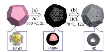
Scheme 1 Schematic illustration of the formation procedure of 3D NCF via calcining ZIF-67 (a), and then etching to remove the Co (b). The figures in the bottom row illustrate the subunit structure of each material.
