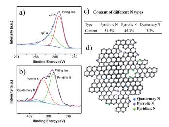
Fig. 3 High resolution XPS spectra for C 1s (a) and N 1s (b). The proportions of each N type (c), and a structural illustration of the carbon shell in NCF (d).
