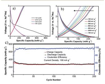
Fig. 5 Sodium storage performance of the NCF: discharge-charge profiles for the first 4 cycles at a current density of 100 mA  $g^{-1}$  (a); rate capability at various current densities (100–2000 mA  $g^{-1}$ ) (b); and cycling performance (c).
