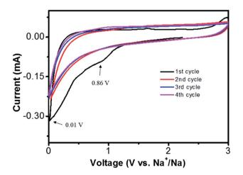
Fig. 4 Cyclic voltammograms of the Na/NCF half cells at 0.5 mV s  $^{-1}$  scan rate, voltage 0.001–3 V.
