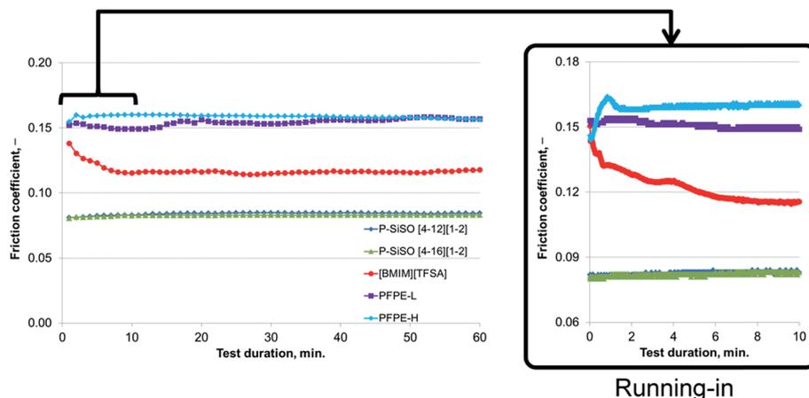
Fig. 3 Friction traces from initial screening tribotests under conditions  $C\{100\text{ N}/25\text{ }^\circ\text{C}/60\text{ min}\}$  (a magnified image corresponding to the running-in period is shown). It can be seen that the friction traces are clearly separated and indicate distinct differences in the running-in behaviors.
