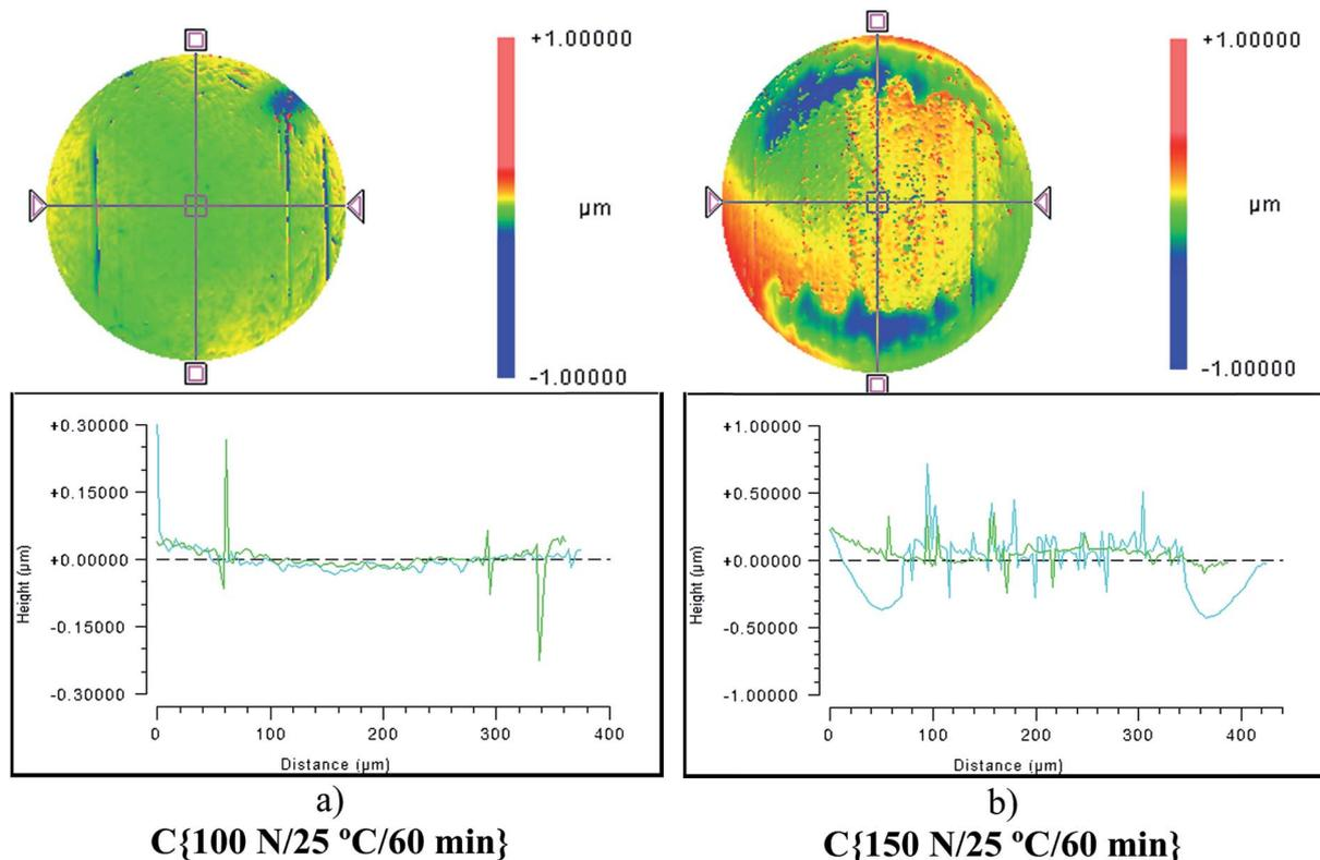
Fig. 7 Surface topography (above) and profilometry (below) of the regions inside the wear scars for P-SiSO[4-16][1-2] after evaluation at different loads. At low load, surface remains very smooth while higher leads to a change in the wear scar morphology.
