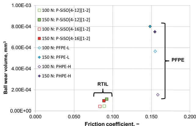
Fig. 5 Ball wear volume versus mean friction coefficient as determined by initial screening tests under conditions of  $C\{100\text{ N}/25\text{ }^\circ\text{C}/60\text{ min}\}$  and  $C\{150\text{ N}/25\text{ }^\circ\text{C}/60\text{ min}\}$ . The P-SiSOs show stable responses to increased loads, unlike the evaluated PFPEs.
