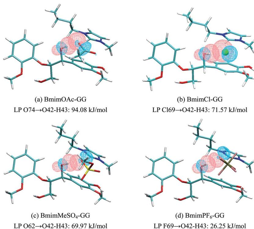
Fig. 5 Natural bond orbital interaction in (a) BmimOAc-GG, (b) BmimCl-GG, (c) BmimMeSO<sub>4</sub>-GG, and (d) BmimPF<sub>6</sub>-GG conformer calculated at B3LYP-D3/6-311+g\*\* level (pink: isovalue = 0.05, blue: isovalue = -0.05).
