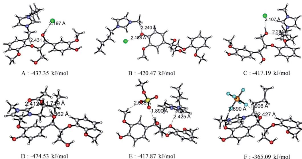
Fig. 4 Optimal structures of interaction between GG and Bmim based ILs at B3LYP/6-31++g\*\* level and H bonds are indicated by dashed line. Structures (A), (B), and (C) are BmimCl–GG interaction at  $\alpha$ ,  $p$ , and  $\gamma$  position respectively. Structures (D), (E) and (F) are BmimOAc–GG, BmimMeSO<sub>4</sub>–GG, and BmimPF<sub>6</sub>–GG interaction at  $\alpha$  position.
