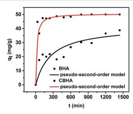
Fig. 8 Adsorption kinetics of CR fitted by pseudo-second-order kinetic model on BHA and CBHA.
