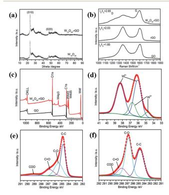
Fig. 3 (a) XRD of  $W_{18}O_{49}$ –rGO composite catalyst. (b) Raman spectra and (c) XPS spectra of GO and  $W_{18}O_{49}$ –rGO composite; (d) high-resolution W 4f spectrum and corresponding deconvoluted spectra of  $W_{18}O_{49}$ –rGO composite; (e) and (f) C 1s core-level and corresponding deconvoluted spectra for  $W_{18}O_{49}$ –rGO composite and GO.
