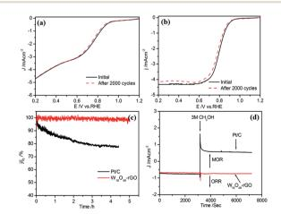
Fig. 5 (a)  $W_{18}O_{49}$ –rGO and (b) Pt/C before and after 2000 potential cycles in  $O_2$ -saturated 0.1 M KOH. The potential was cycled between 0.2 and 1.2 V at a rate of 50 mV s $^{-1}$ . (c) Chronoamperometric response of  $W_{18}O_{49}$ –rGO and Pt/C. (d) Chronoamperometric response of  $W_{18}O_{49}$ –rGO and Pt/C before and after addition of 3 M methanol. The tests were conducted in  $O_2$ -saturated 0.1 M KOH solution at 0.70 V.
