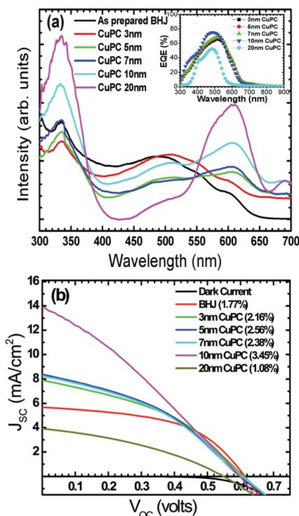
Fig. 1 (a) UV-visible absorption spectra of copper phthalocyanine buffer layers in respect of their thickness; inset shows EQE analysis. (b) Shows  $J$ - $V$  characteristics of corresponding bulk-heterojunction solar cells.
