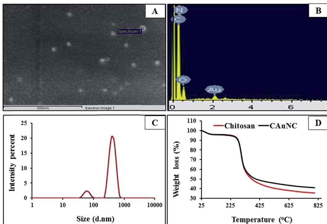
Fig. 2 FE-SEM image, particle size and thermal stability of CAuNC. (A) FE-SEM image; (B) EDX spectra; (C) particle size distributions of CAuNC solution in 0.25% acetic acid; (D) thermograms of chitosan and CAuNC.
