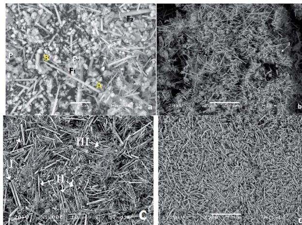
Fig. 8 LV-SEM micrographs showing the products obtained in the synthesis of HAp by hydrothermal process at (a) 230  $^{\circ}\text{C}$  for 20 h, (b) 250  $^{\circ}\text{C}$  for 20 h, (c) 230  $^{\circ}\text{C}$  for 48 h and (d) 250  $^{\circ}\text{C}$  for 48 h.
