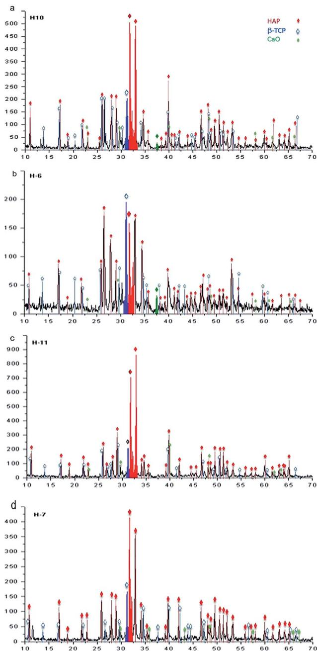
Fig. 9 X-ray spectra associated with the hydrothermal synthesis using a stoichiometric concentration ratio of 3 : 1 of  $\beta$ -TCP : CaO for 20 h at (a) 230 °C, (b) 250 °C, and for 48 h at (c) 230 °C and (d) 250 °C.
