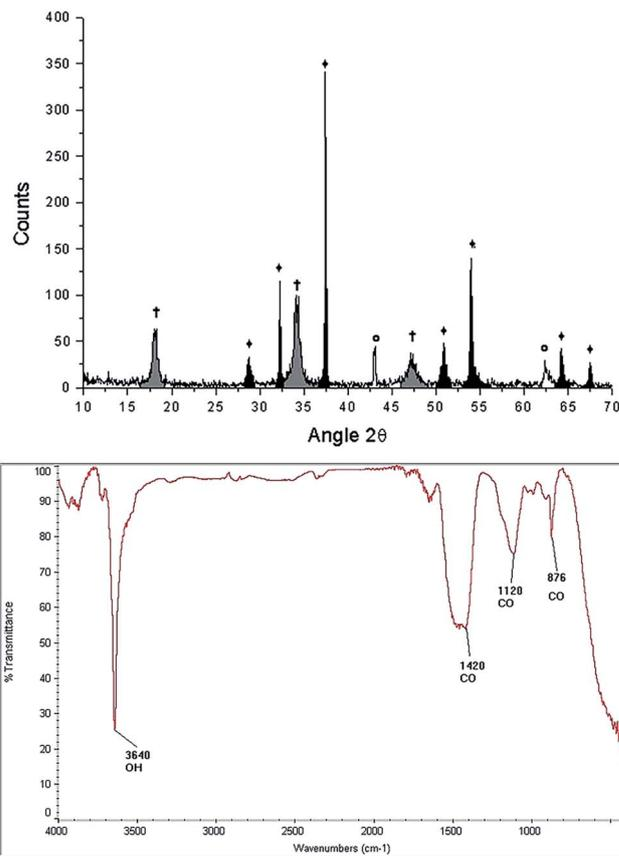
Fig. 5 Characterization of the starfish *Mellita eduardobarrosi* sp. nov. after the thermal treatment: diffractogram (up) showing the phases: †[Ca(OH)<sub>2</sub>], ♦[CaO], ⊙[MgO], and FTIR spectrogram (bottom).
