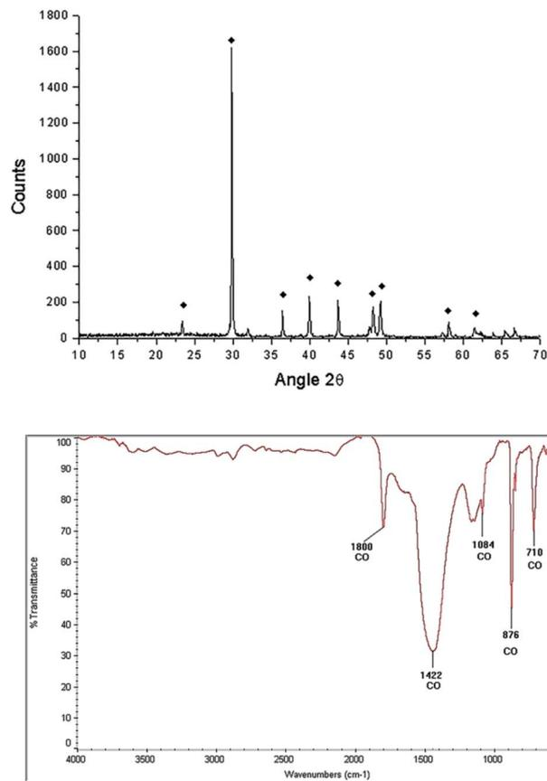
Fig. 4 Characterization of the starfish *Mellita eduardobarrosi* sp. nov.: diffractogram (upper panel), black marks represent the predominant phase which corresponds to magnesium calcite, and FTIR spectrogram (lower panel).
